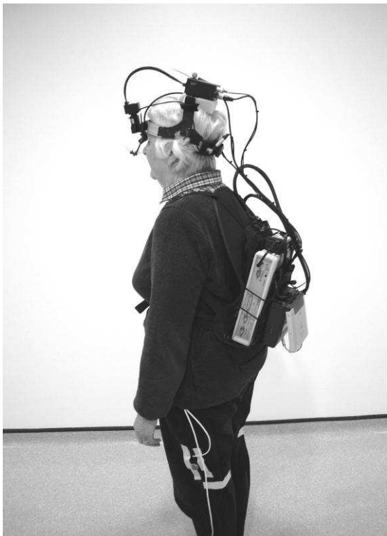
Figure 2.1: OA with mobile eye-tracker and attached LED light to detect foot contact on the stair
