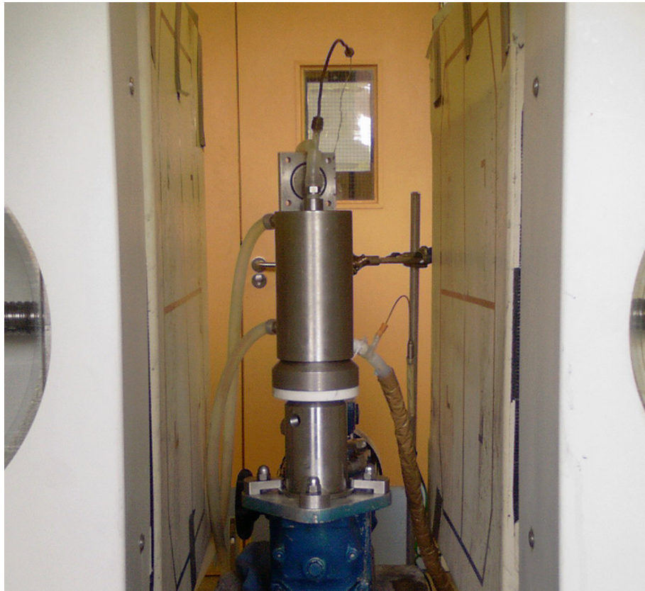
Figure 3.5: The pin stirrer within the PEPT cameras
