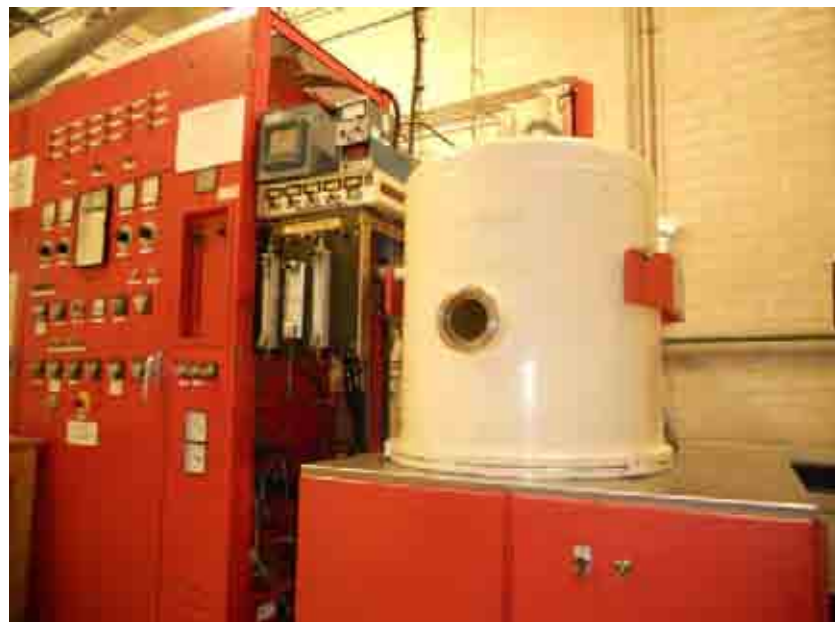
Figure 3.2-1 The 40kW Klöchner Ionon GmbH plasma unit at the University of Birmingham DC plasma vacuum unit
