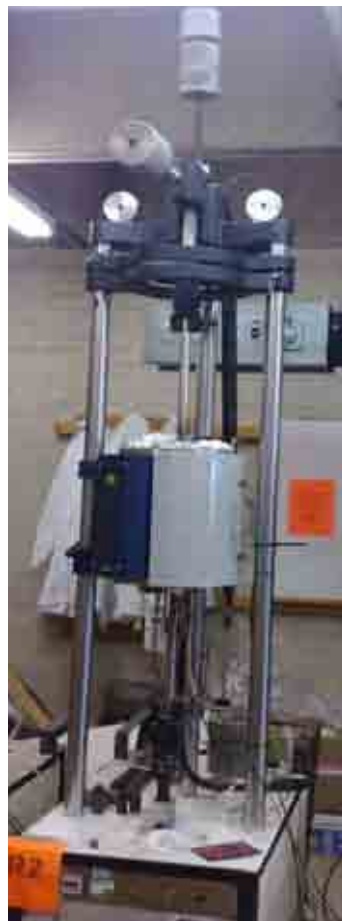
Figure 3.2-6 Installations for experiments of annealing of carburised 316ASS under tensile stresses
