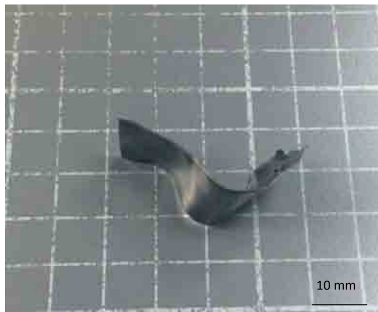
Figure 4.1-1 The picture of 316L foil specimen after plasma carburising
