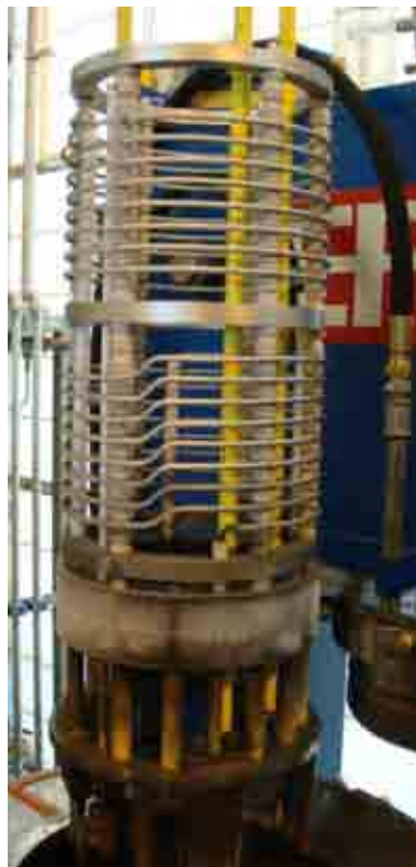
Figure 3.2-4 The molybdenum furnace of HIP facility at the University of Birmingham
