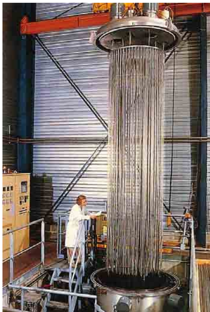
Figure 2-8 Plasma treatment of control rod cluster of AISI 316 tubes for nuclear reactor [6]
