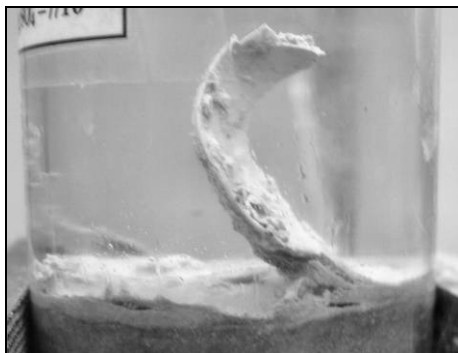
Figure 4.5 - Mix 3 (290-0.75) sample after 7 months in \text{SO}_4 -solution, side view
