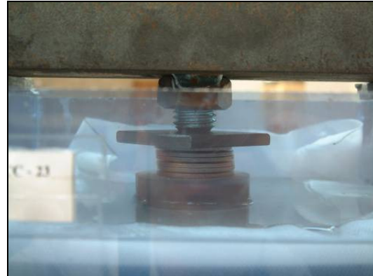
Figure 3.14 - Disc spring arrangement
