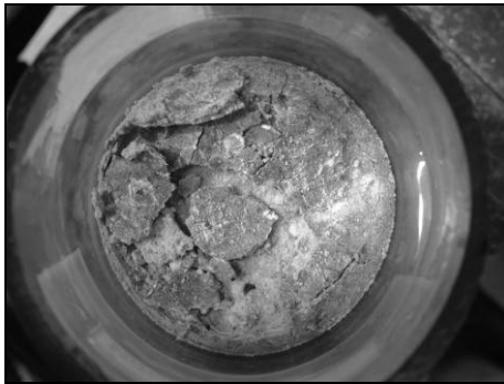
Figure 4.19 - Mix 3-CS (290-0.75) sample after 15 months in \text{SO}_4 -solution, top view
