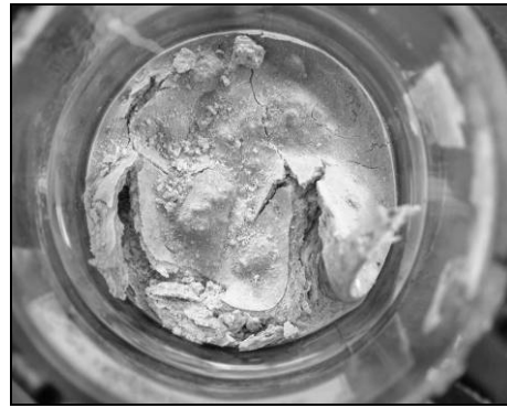
Figure 4.4 - Mix 3 (290-0.75) sample after 9 months in \text{SO}_4 -solution, top view
