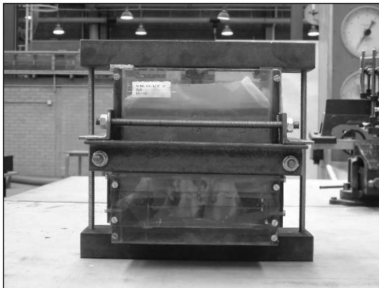
Figure 3.9 - Shear test specimen with pressure frame
