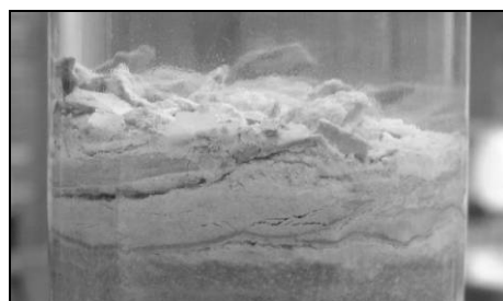
Figure 4.8 - Mix 3 (290-0.75) sample after 27 months in \text{SO}_4 -solution, side view
