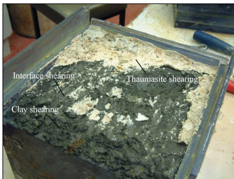
Figure 5.28 - Combined interface shear plane, clay view
