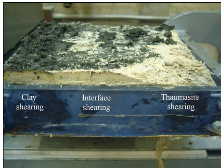
Figure 5.29 - Combined interface shear plane, concrete view
