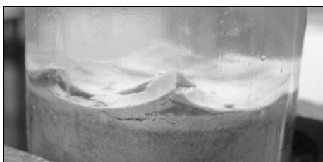
Figure 4.7 - Mix 3 (290-0.75) sample after 7 months in \text{SO}_4 -solution, side view
