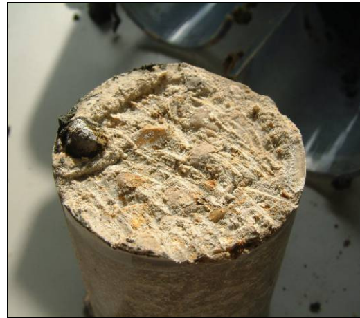
Figure 5.6 - Thaumasite layer at precast - LLC, after sampling
