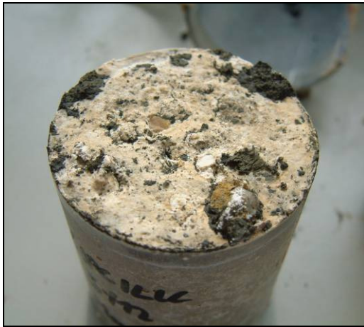
Figure 5.5 - Thaumasite layer at precast - LLC
