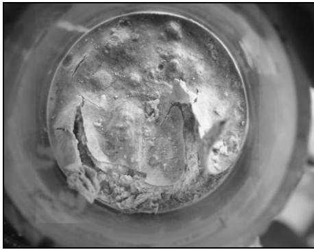
Figure 4.3 - Mix 3 (290-0.75) sample after 7 months in \text{SO}_4 -solution, top view
