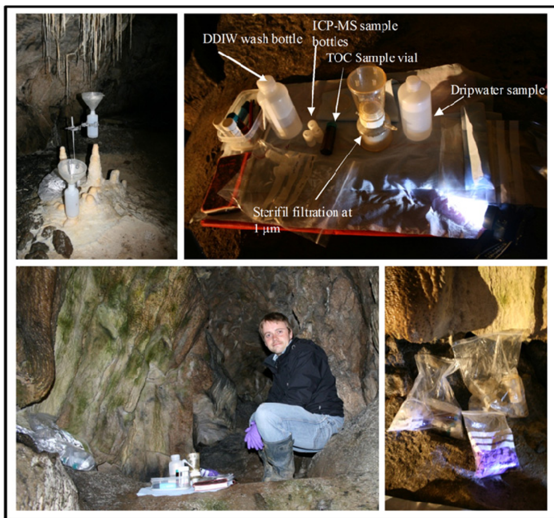
Figure 3.3 Images of fieldwork at Poole’s Cavern, Buxton, UK. Clockwise from top left: sampling of dripwater in Roman Chamber, “field-laboratory” setup, field supplies in clean plastic bags, the author during sampling.
