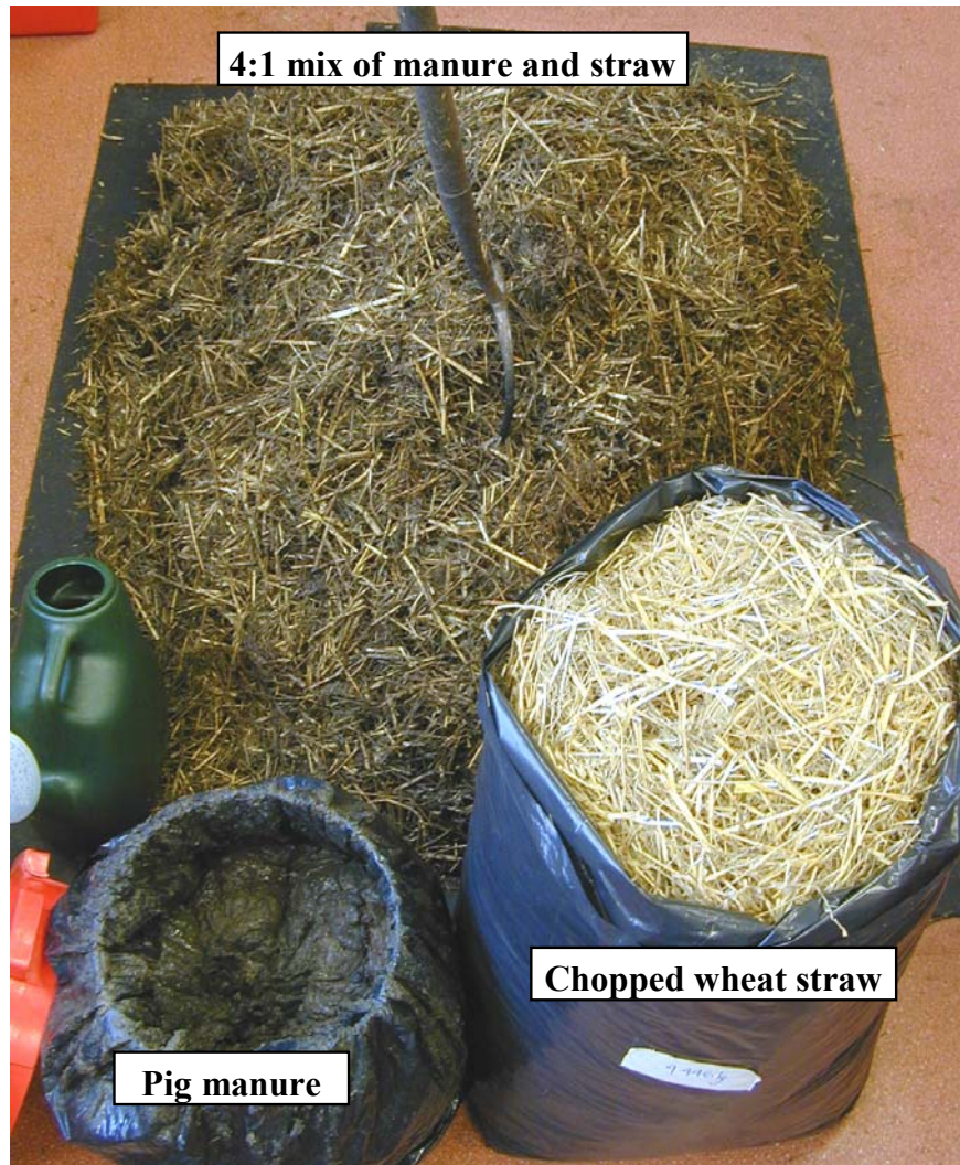
Figure 3.14. The pig manure and straw before and after mixing in the ratio of 4
