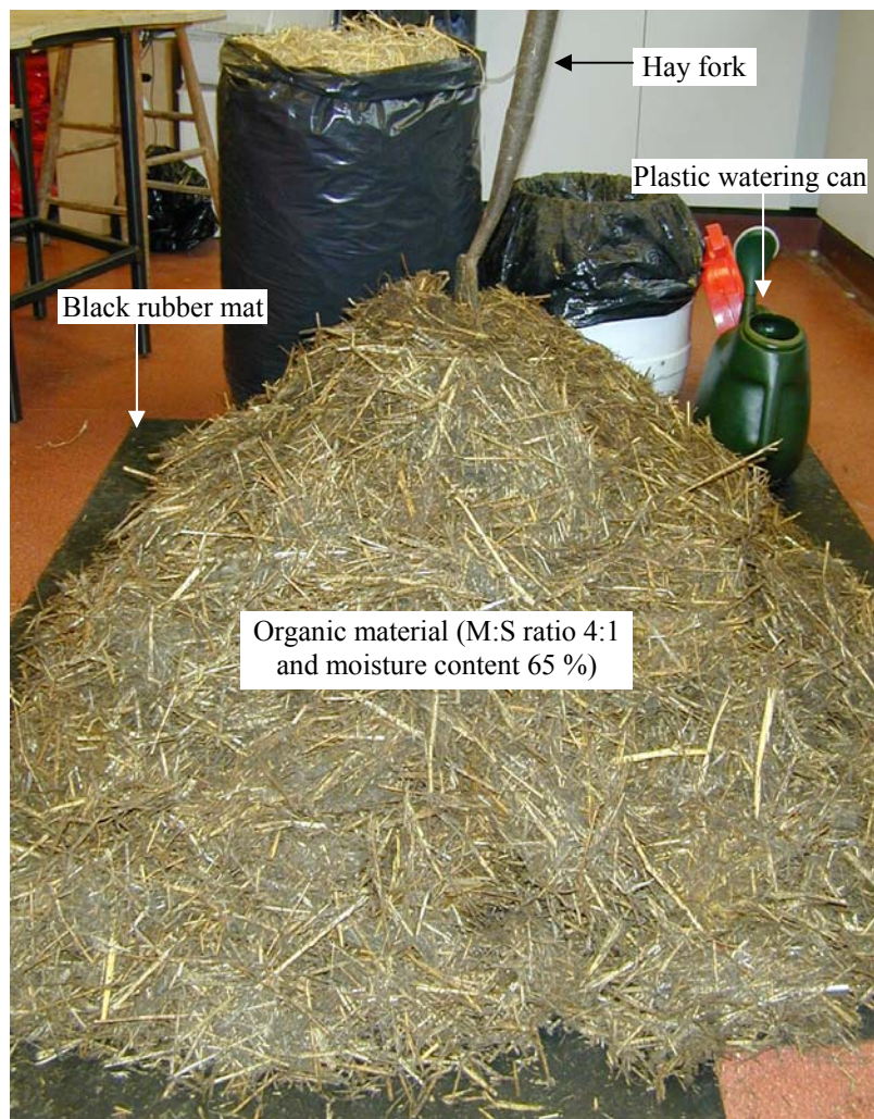
Figure 6.3. Approximately 47 kg of the organic material ready for loading into the reactors.
