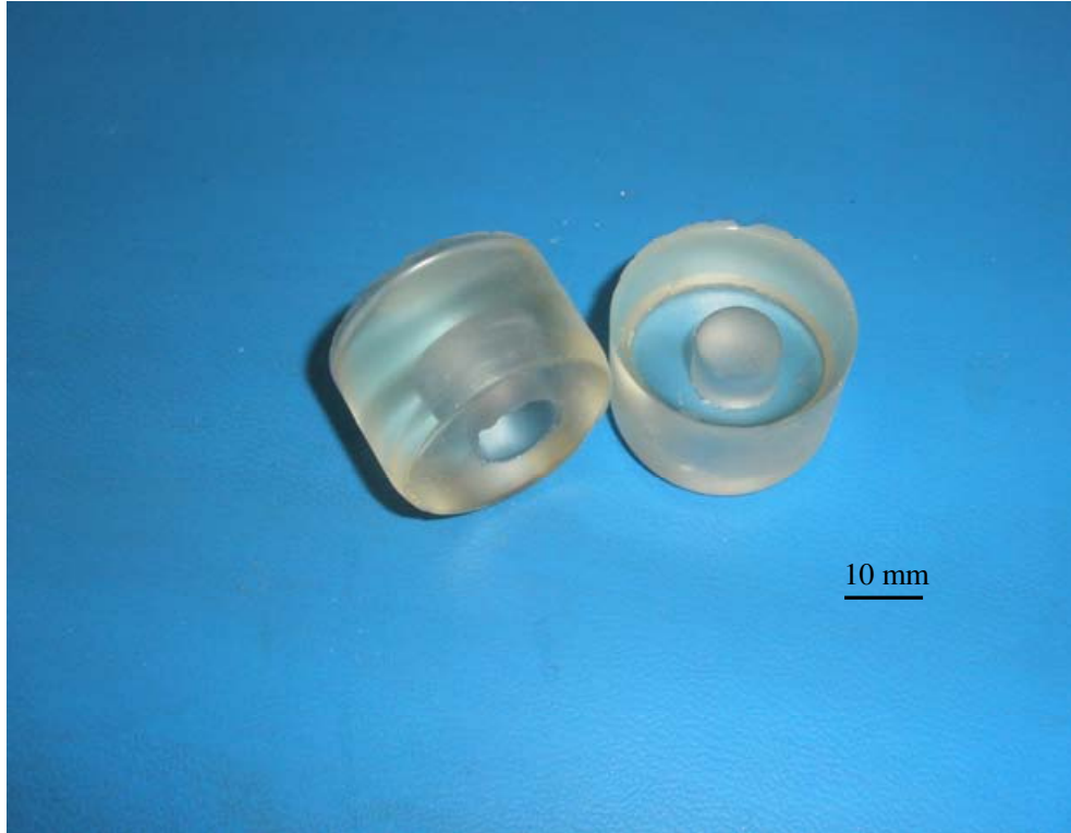
Figure 3.2 Typical PDMS moulds used in this study
