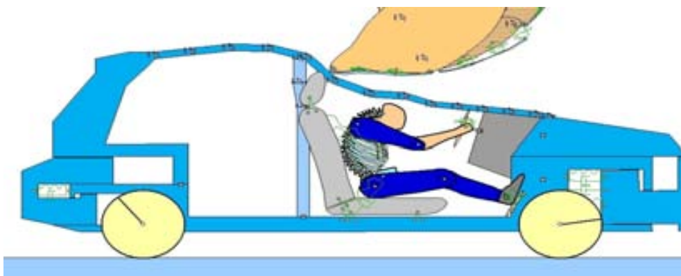
Figure 8.56: Snapshots from the simulation of the Case I crash showing the contact of the camel with the vehicle
