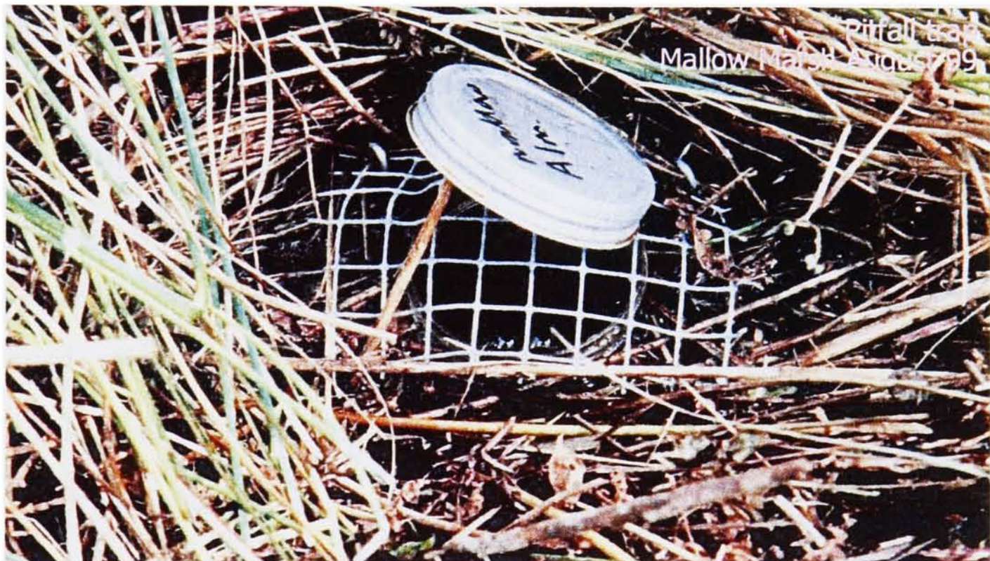
Figure 1.14 The shrew excluder was highly effective at preventing small mammal, amphibians and lizards from drowning in the pitfall traps.
