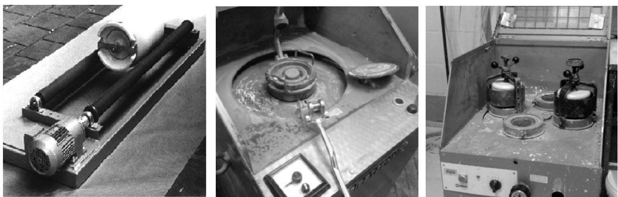
Figure 4-1: Different types of laboratory milling machines used in the experiments; from left to right: ball mill, ring mill and planetary mill
