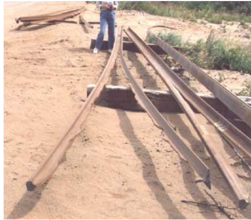
Figure 2.5: A rail broken along the web of the rail due to high residual stress (Igwemezie 2007, p. 2)
