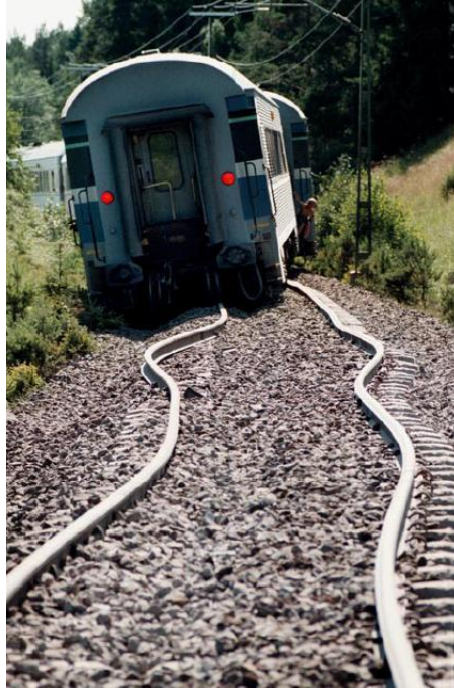
Figure 2.1: Train derailed by a buckled rail in Sweden (Photo: Frida Hedberg, Aftonbladet Bild)
