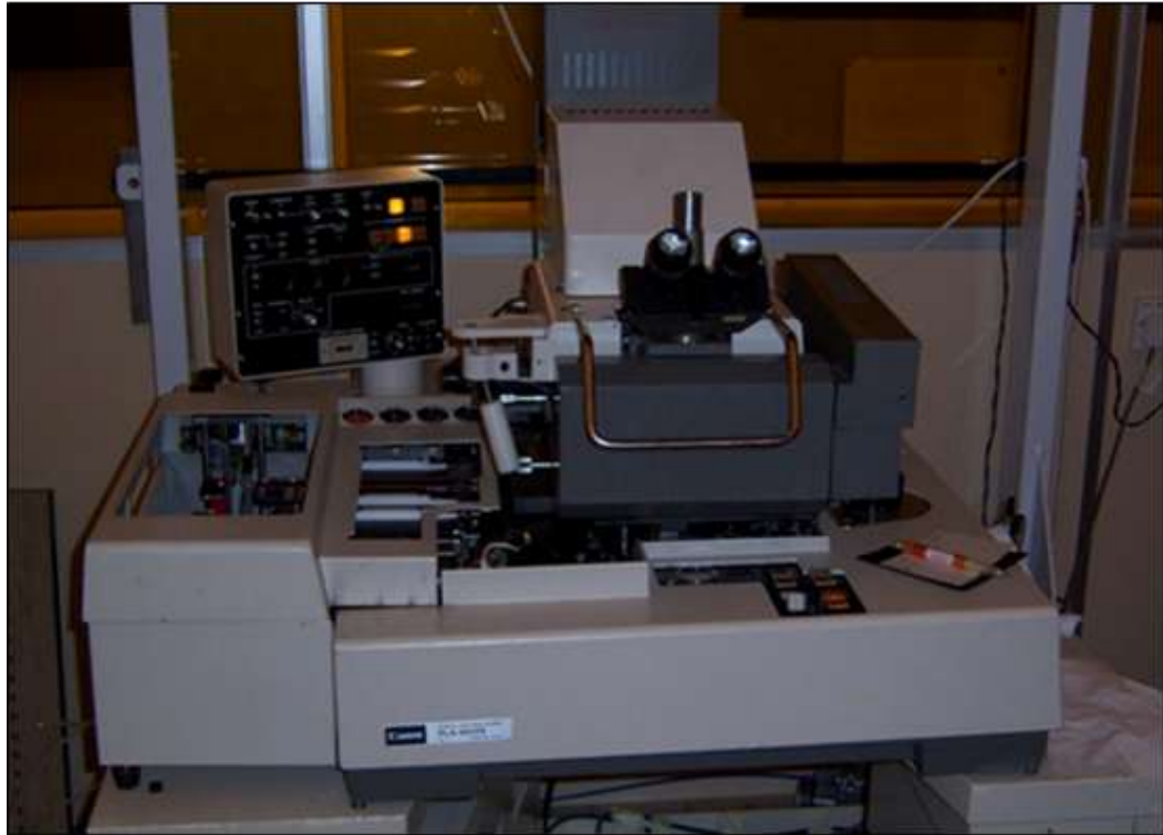
Figure 3.4. A photograph showing a Cannon PLA-501 mask aligner machine used for exposing the SU-8 by UV-light.
