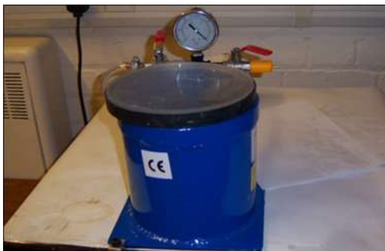
Figure 3.12. A photograph showing the degassing chamber used in this research.
