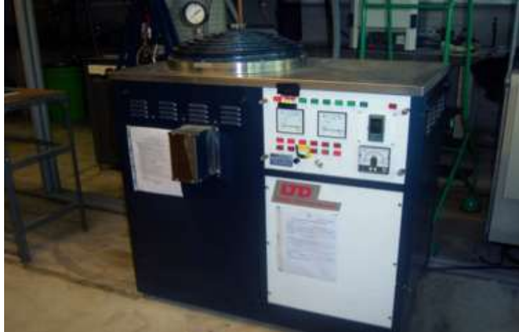
Figure 6.5. A photograph showing the vacuum furnace used for sintering stainless steel micro components under vacuum atmosphere.
