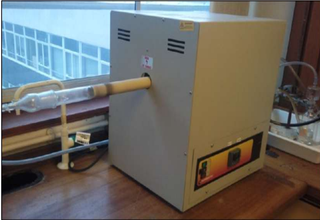
Figure 6.4. A photograph showing a tube furnace used for de-binding and sintering stainless steel micro components under nitrogen/hydrogen mixture atmosphere.
