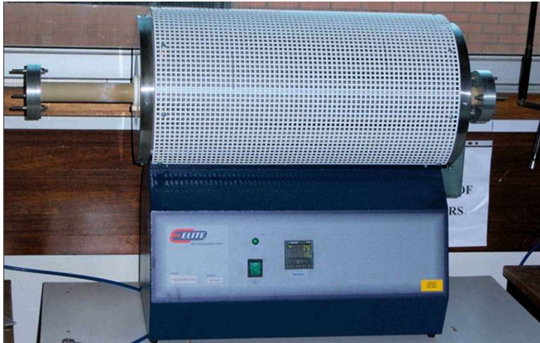
Figure 6.3. A photograph showing the tube furnace used for de-binding and sintering stainless steel micro components under nitrogen atmosphere.
