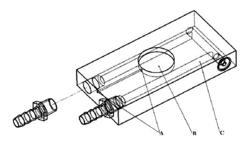
**Figure 5.** Aluminium block design used to measure aphid activity thresholds. A. channel for the thermocouple to measure arena temperature; B. Aphid arena; C. Channel for pumping alcohol fluid to enable fine temperature control over the arena (Hazell *et al.*, 2008).
