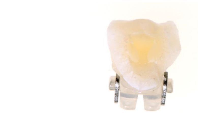
Figure 4.2 Sample 8, Group 3 – fractured labial enamel with bonded Clarity© bracket in situ
