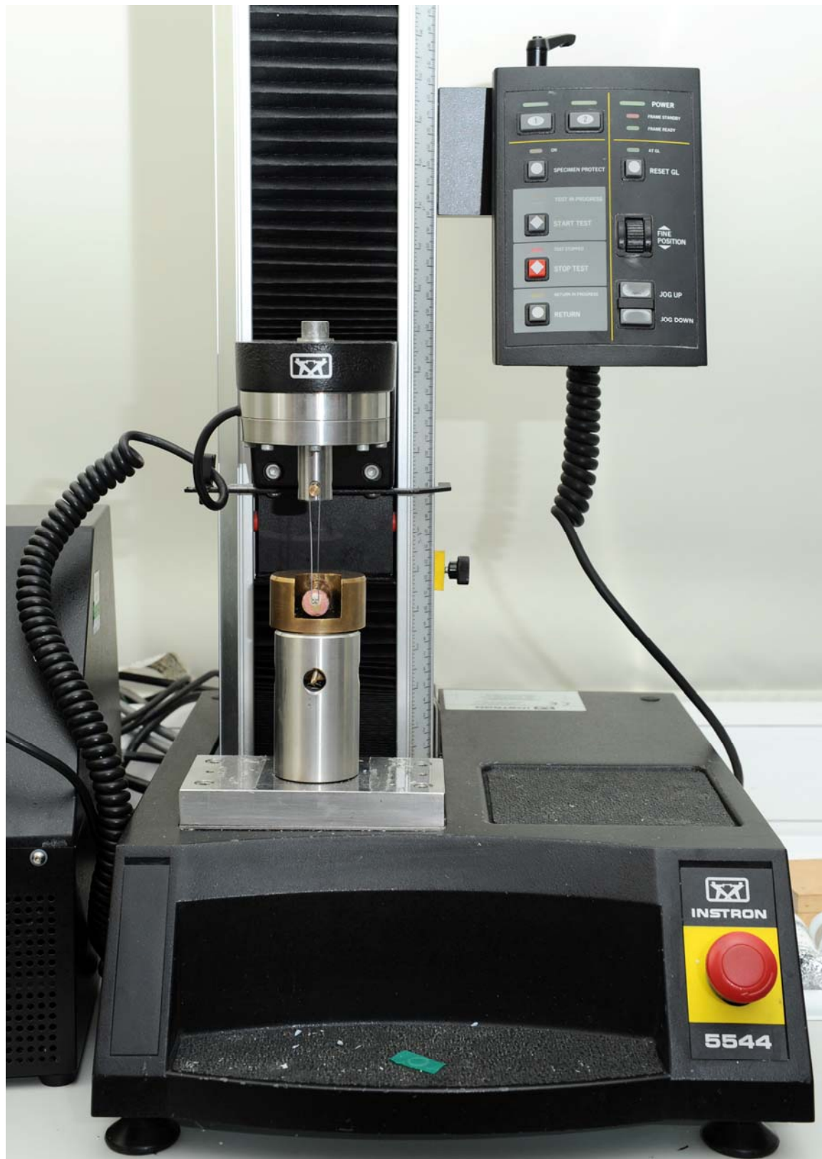
Figure 2.1 Laboratory set-up: Instron Universal Testing Machine
