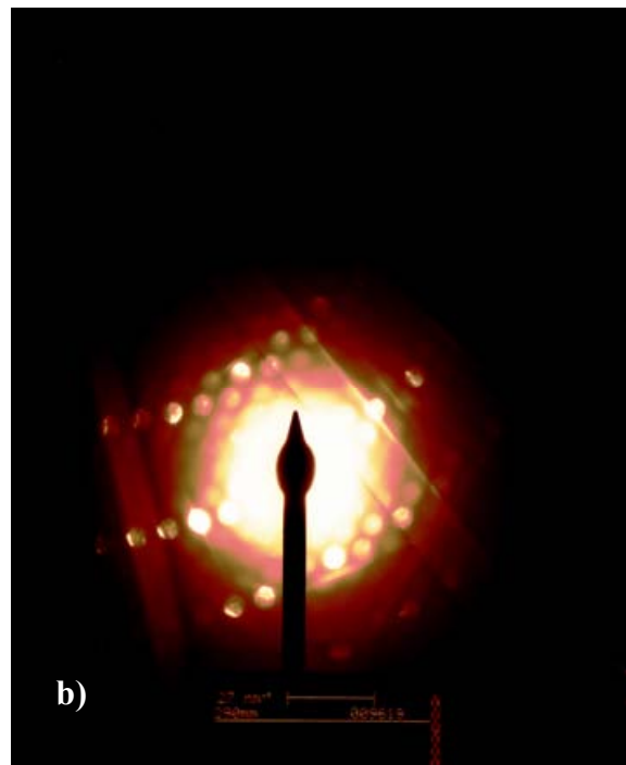
Figure 4.4. TEM Study: AA2096 UA4 Temper. Area 1. CBED.
