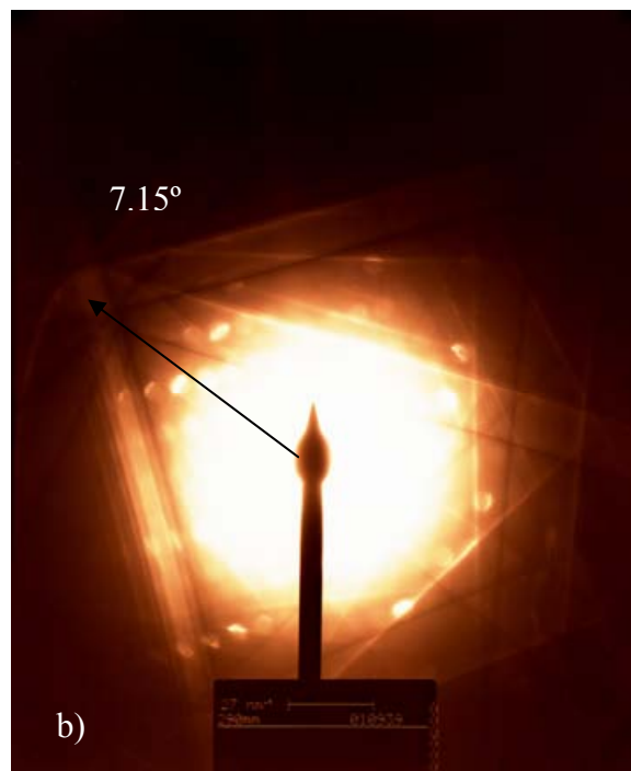
Figure 4.38. TEM Study: AA2096 UA12 Temper. CBED.
