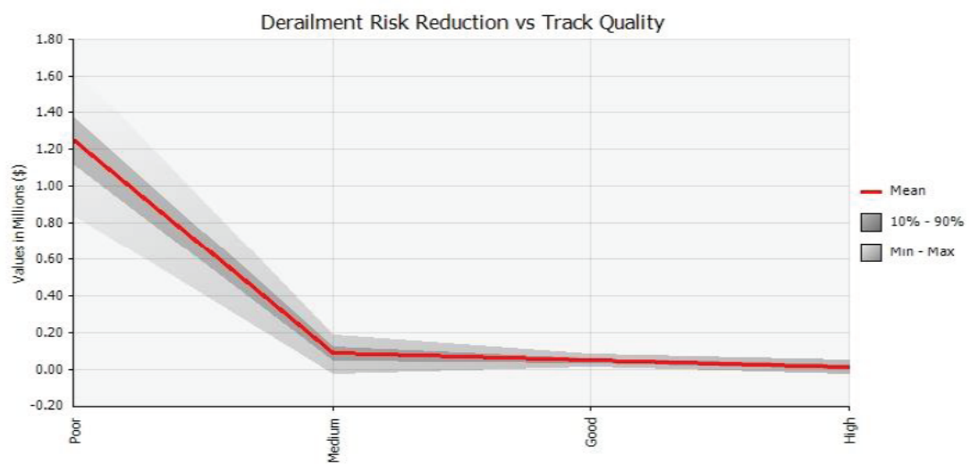
Figure 5(c) Derailment Risk reduction by upgrading Track Quality on the Iron Ore Line in Sweden
