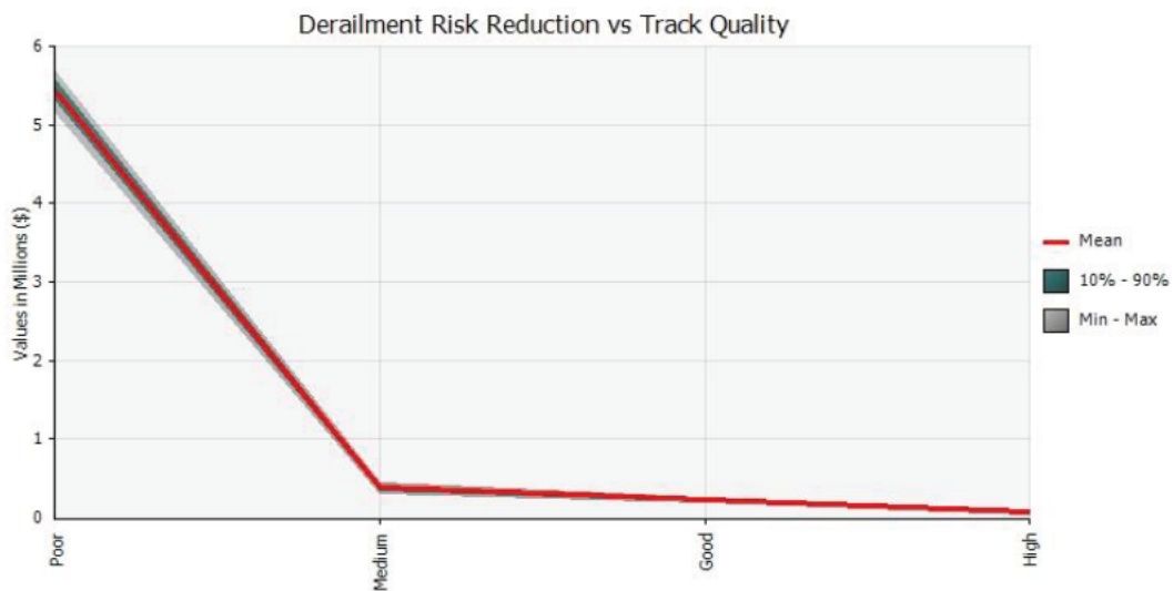
Figure 7(c) Derailment Risk reduction by upgrading Track Quality on the Trans-Australian Route
