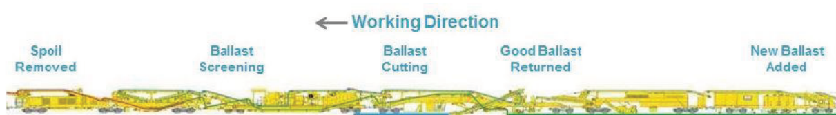
Figure 6.14 High Output Ballast Cleaning System operated by Network Rail (Source: Network Rail)
