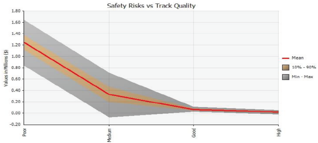
Figure 5(b) Safety Risk of Derailments vs Track Quality on the Iron Ore Line in Sweden
