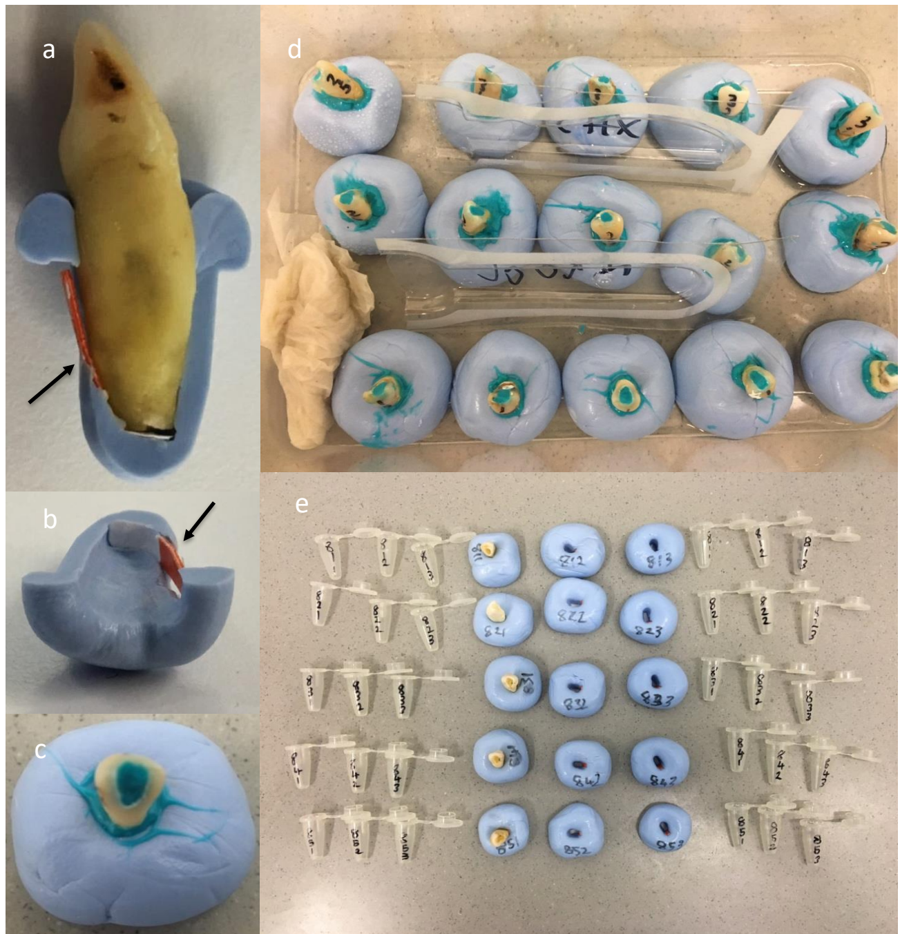
Figure 7: Photographs of the experimental set up used in experiment 3.4. (a & b) cross sectional views of the tooth apex in contact with the PerioPaper (OraFlow, New York, USA); which is marked with a black arrow and mounted in a putty base putty (Henry Schein, NY, USA) (c & d) groups with \text{Ca(OH)}_2 paste (UltraCal, Ultradent, USA) kept in a container with an incubator (not shown) and the access cavities sealed with light bodied silicone (Henry Schein, NY, USA ) (e) multiple putty bases for the teeth to be moved during each 5 minute irrigation with the secondary irrigant.
