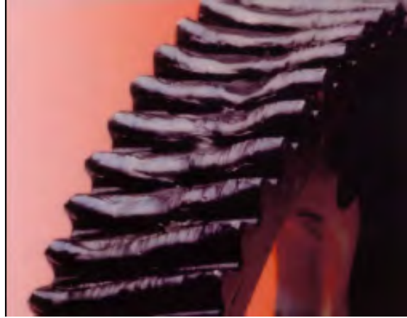
Figure 3.23: An example of plastic flow defect [69].
