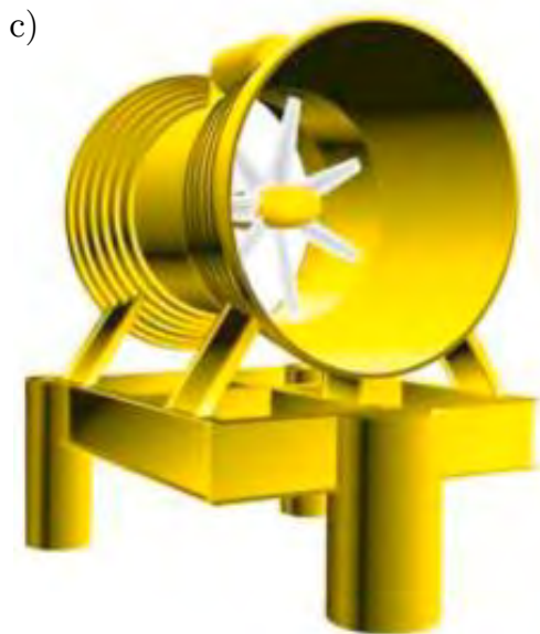
Figure 2.1: Different types of tidal turbines; a) Horizontal axis; b) Polo turbines; c) Venturi (duct) effect; d) Horizontal axis [16–18]
