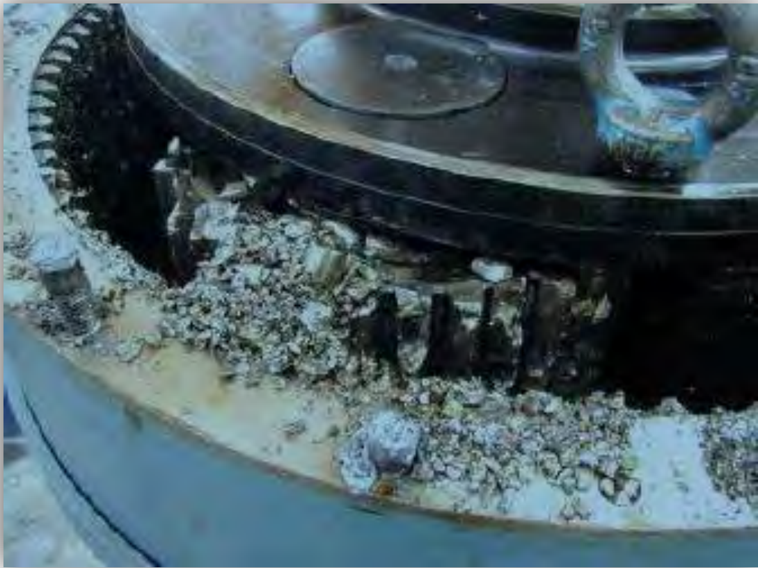
Figure 3.1: Broken planetary gear in gearbox. Figure taken from [34].
