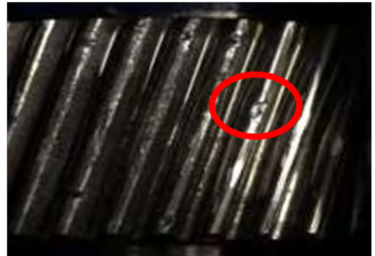
Figure 5.10: Inducing small chips on the gear teeth.
