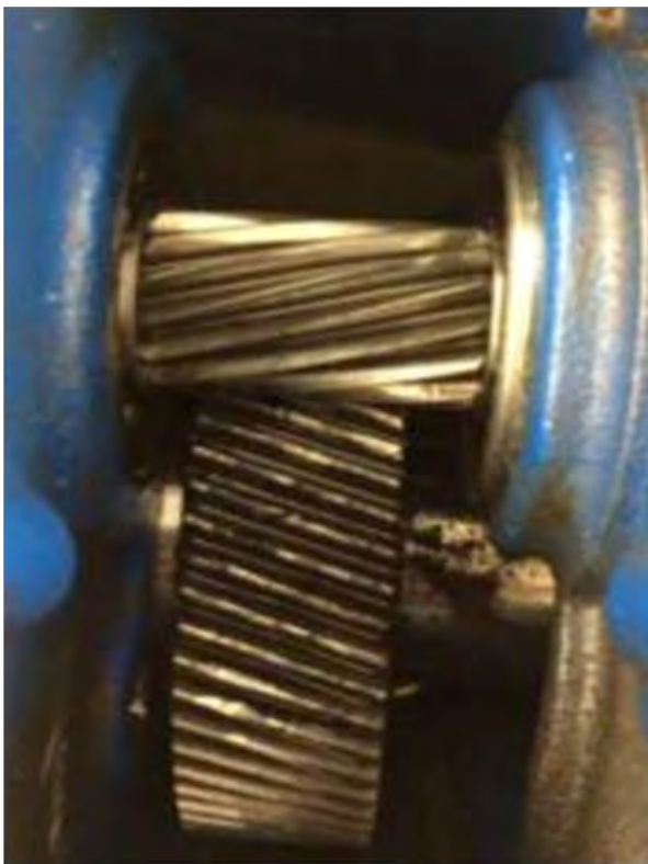
Figure 5.10: Inducing small chips on the gear teeth.
