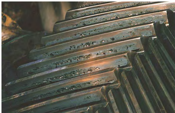
Figure 3.22: Gear tooth pitting [67].
