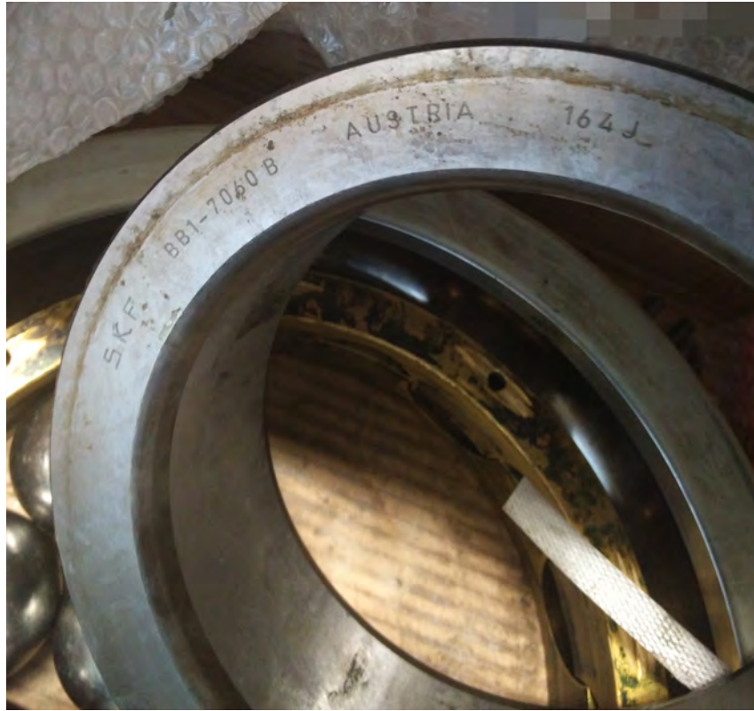
Figure 6.16: The removed generator bearing from M1 wind turbine.
