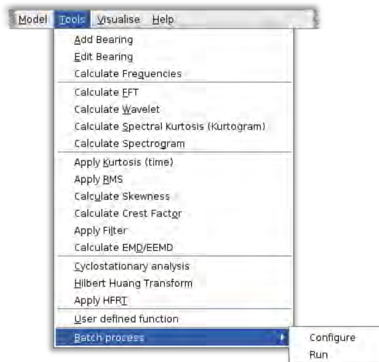
Figure 7.7: The tools menu showing various signal processing techniques available to the user.
