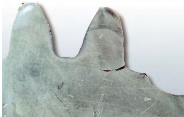
Figure 3.17: Gear tooth breakage [66].
