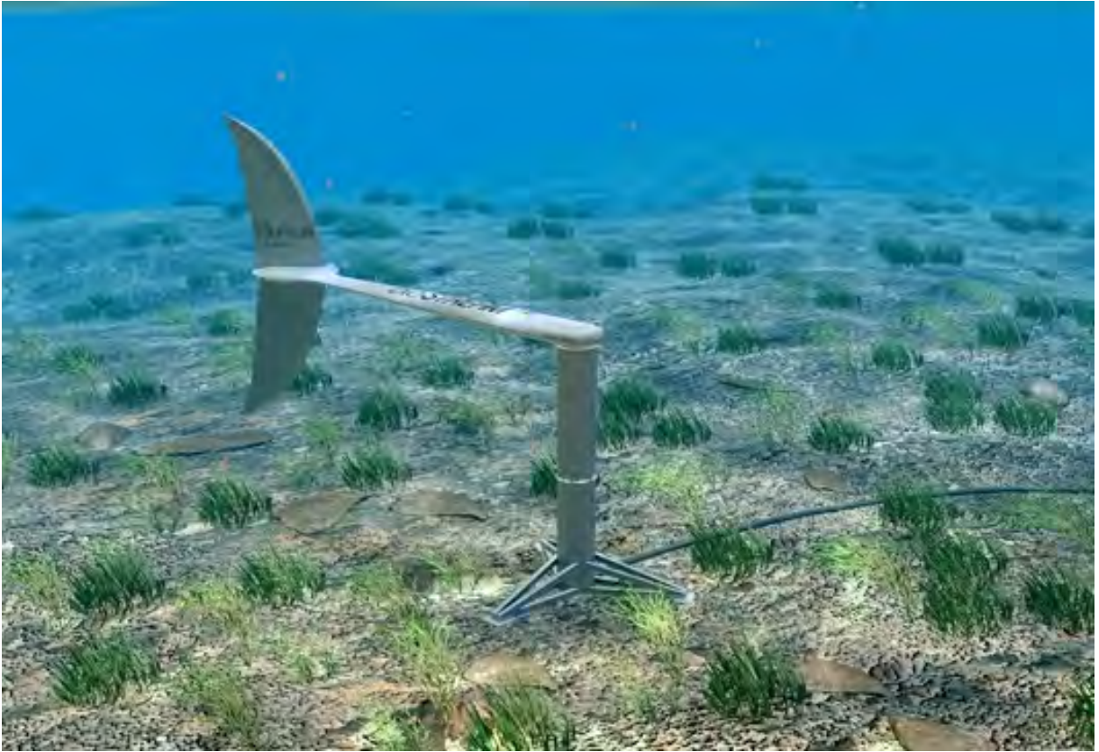
Figure 2.2: Oscillatory-hydrofoil turbine concept, developed by BioPower System company [17]
