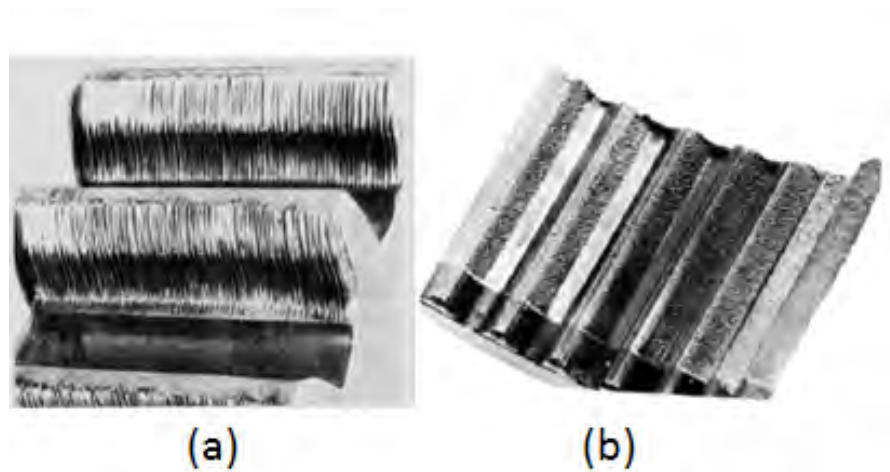
Figure 3.21: Corrosive wear or chemical wear [64].
