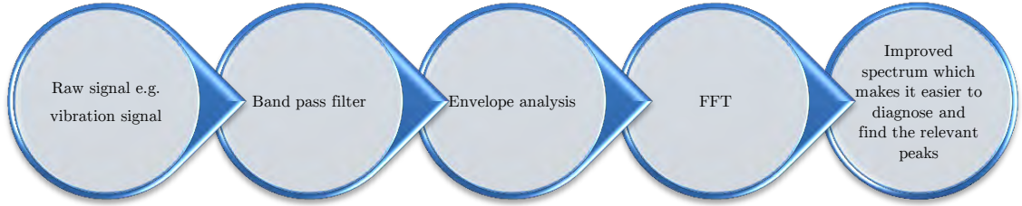
Figure 4.9: High Frequency Resonance Technique algorithm.
