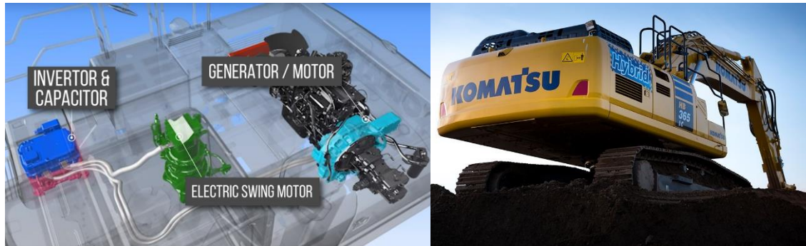
Fig. 1-10 Hybrid swing system of Komatsu's excavator ( Komatsu Hybrid Technology, 2019 )
