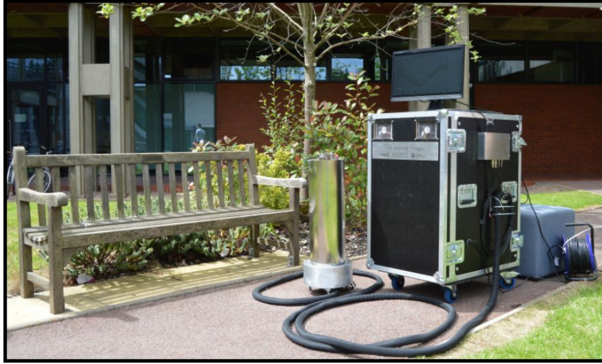
Figure 2.16: The gravimeter prototype in its first foray outdoors to what has become the preliminary testing ground for all portable systems.
