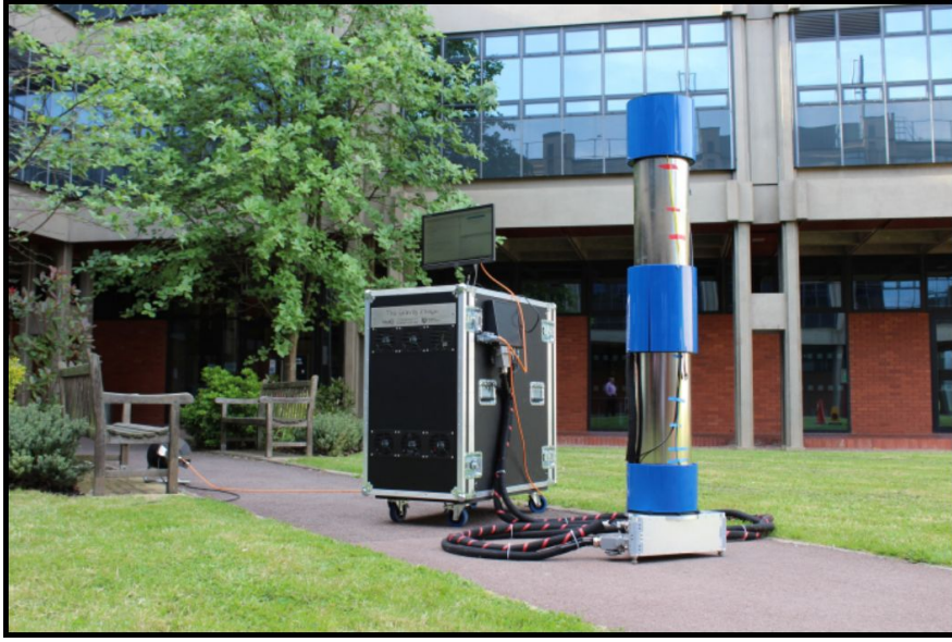
Figure 1.6: The subject of this thesis, the portable gravity gradiometer constructed at the University of Birmingham in its intended environment.
