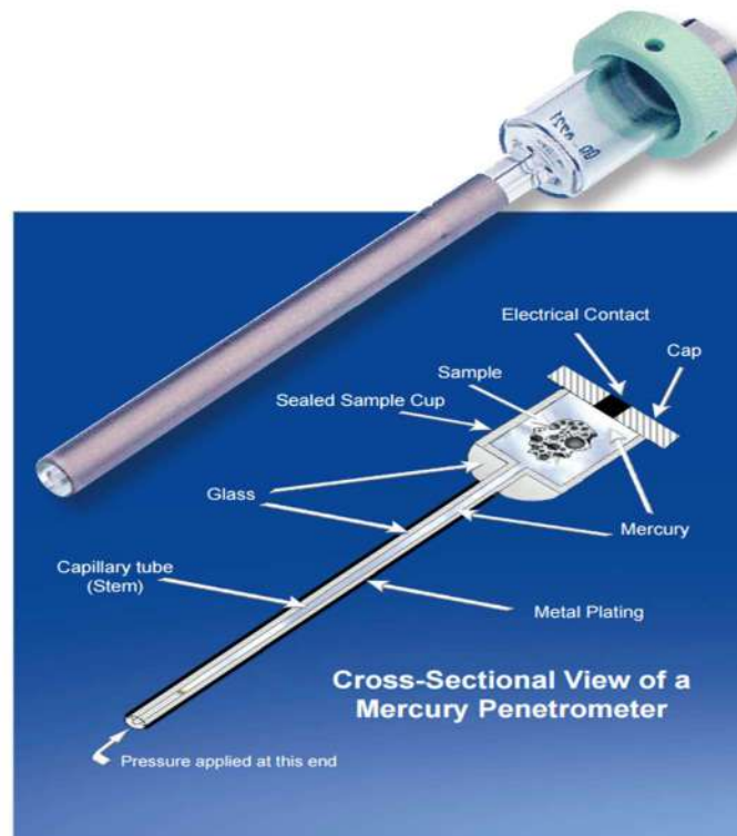
Figure 4. 14: Schematic of a Mercury Intrusion Penetrometer [239]
