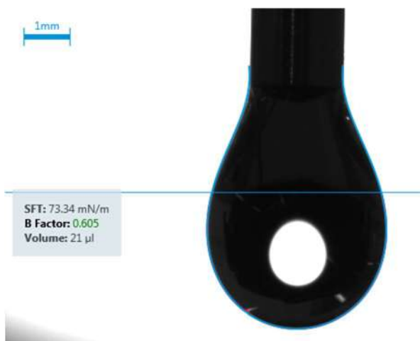
Figure 2. 11: Shape of an amino acid solution drop analysed by the shape analyser software
