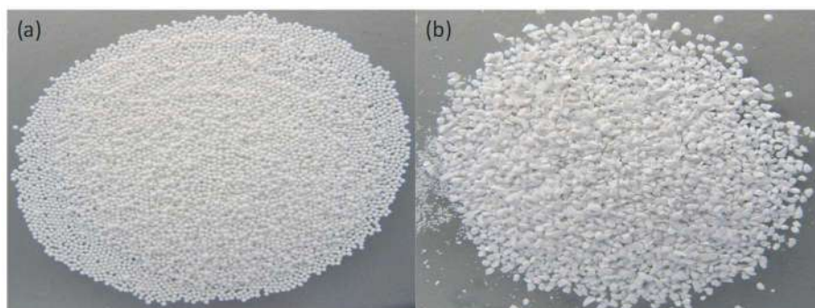
Figure 4. 18: Supports used in FTS test: (a) conventional titania spheres (b) titania foam
