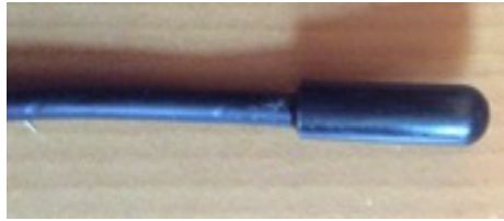
Figure 4-5: Waterproof (DS18B20) probe used to measure soil temperature.
