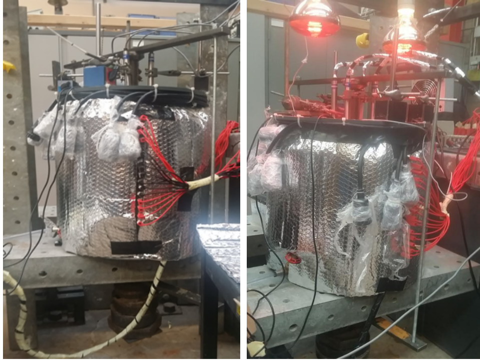
Figure 4-17: Photograph of the test setup; (left) test in laboratory conditions (without heat and breeze), (right) test with heating and breeze sources.
