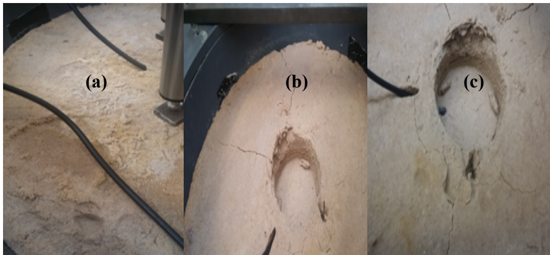
Figure 5-18: Photographs of the soil surface before and after the failure for Case 2; (a) salt over the soil surface when water approached the upper layer, (b) and (c) punching shear and cracking around the footing model.
