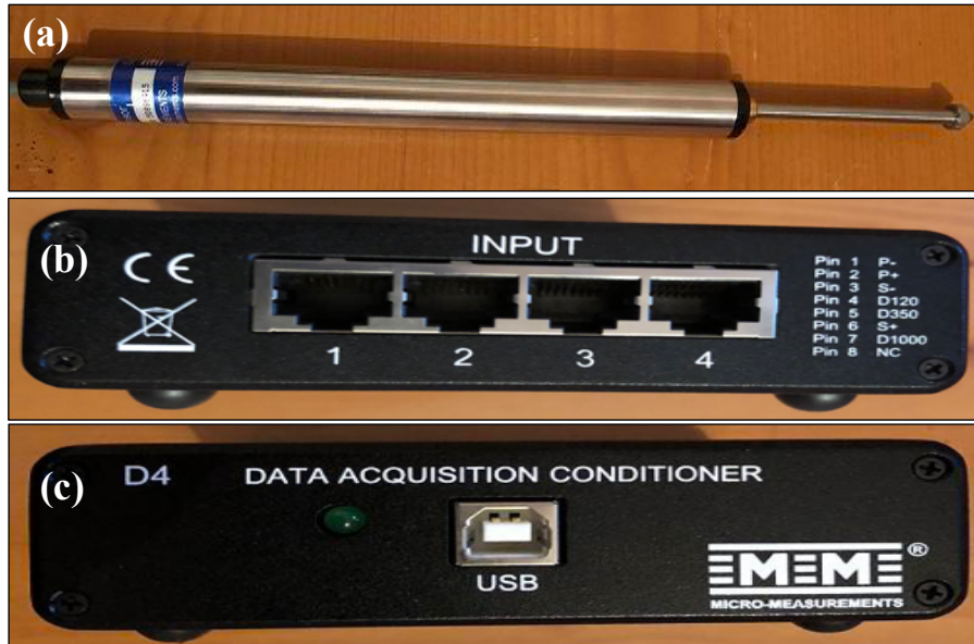
Figure 4-14: (a) Linear displacement sensor (LDS) to measure vertical displacement of footing, (b) The four channels connection side, (c) USB connection attached to the PC via a cable.
