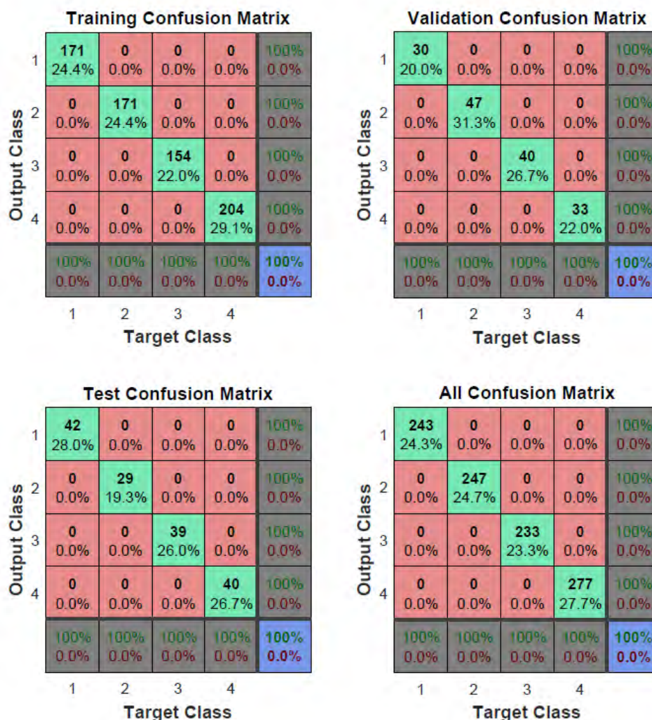
Figure A.2.10 Confusion Matrix Results for 2002 in Legal Maranhão. Accuracy measure using Hansen et al. (2013) dataset. Final confusion matrix is at the bottom right. The rows correspond to the predicted class and the columns correspond to the true class. The diagonal cells correspond to observations that are correctly classified. Both the number of observations and the percentage of the total number of observations are shown in each cell. The column on the far right of the plot shows the percentages of all the examples predicted to belong to each class that are correctly and incorrectly classified. The row at the bottom of the plot shows the percentages of all the examples belonging to each class that are correctly and incorrectly classified. The cell in the bottom right of the plot shows the overall accuracy (MATLAB, 2017).
