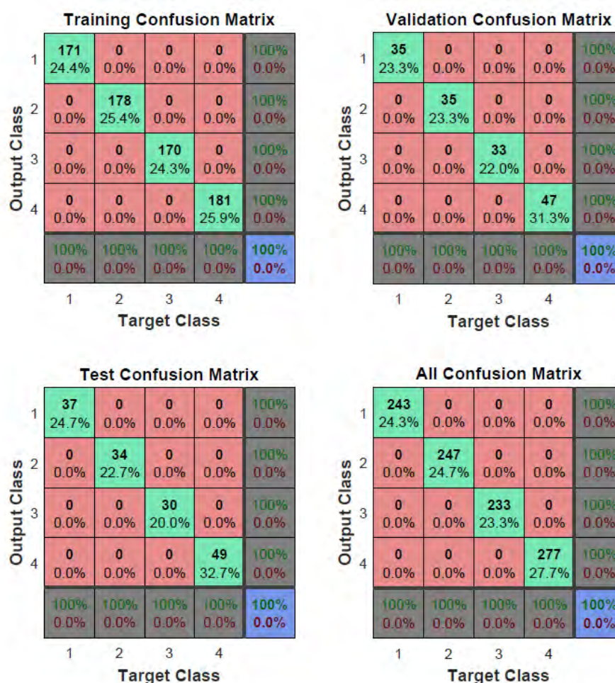
Figure A.2.12 Confusion Matrix Results for 2012 in Legal Maranhão. Accuracy measure using Hansen et al. (2013) dataset. Final confusion matrix is at the bottom right. The rows correspond to the predicted class and the columns correspond to the true class. The diagonal cells correspond to observations that are correctly classified. Both the number of observations and the percentage of the total number of observations are shown in each cell. The column on the far right of the plot shows the percentages of all the examples predicted to belong to each class that are correctly and incorrectly classified. The row at the bottom of the plot shows the percentages of all the examples belonging to each class that are correctly and incorrectly classified. The cell in the bottom right of the plot shows the overall accuracy (MATLAB, 2017).
