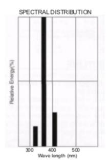
Figure 3.14: Spectral distribution of the 4 W UV lamp used to irradiate analogue 102.
