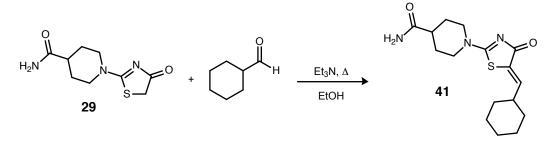
Scheme 2.5: Final step in the synthesis of inhibitor 41.
