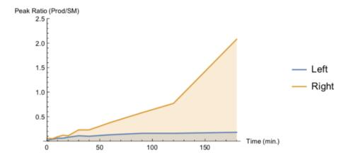
Figure 3.16: Ratio between product formation and impurity used as an internal standard when irradiating diazirine 102 with UV light. Legend term *left* corresponds to the internal standard and *right* to the products formed upon irradiation.
