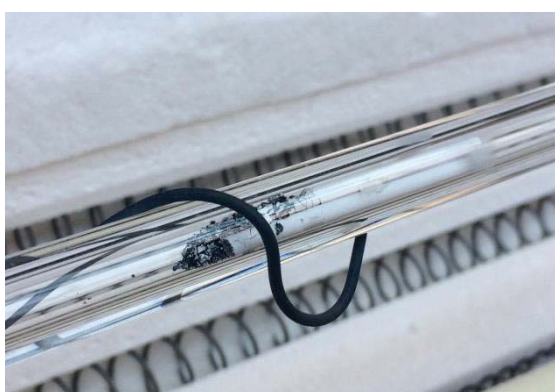
Figure 100: Disintegrated Ni@SiO 2 fibre after testing.
