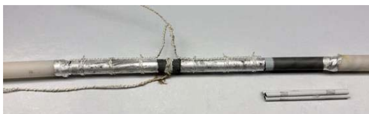
Figure 108: Alumina fibre reactor removed from the fuel cell after testing.
