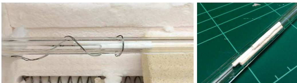
Figure 92: Photographs of fibre reactors held in quartz tubes and showing the position of thermocouple.
