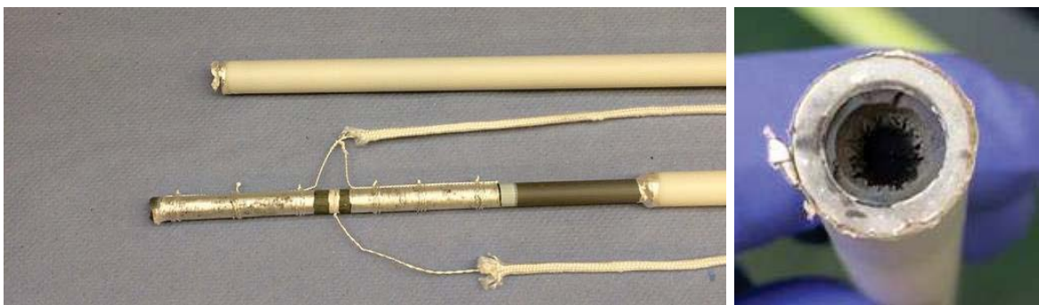
Figure 110: Fuel cell which has been tested on methane. Left: fuel cell fractured away from the manifold Right: blocked fuel cell tube due to carbon deposition.
