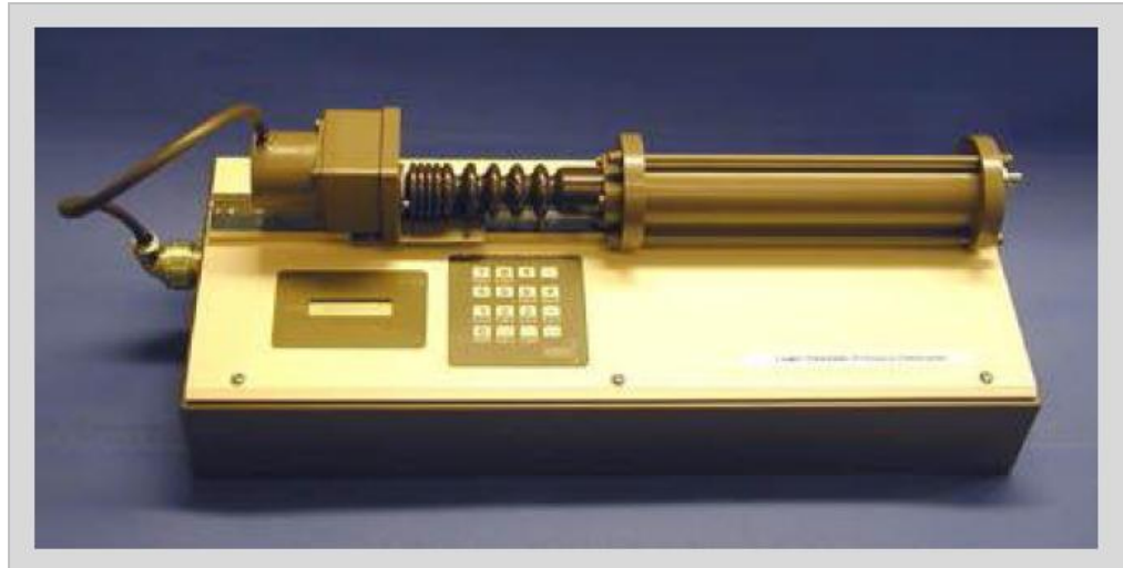
Figure 3.4: The standard hydraulic pressure or volume controller by GDS Instruments (GDS Instruments, 2009)
