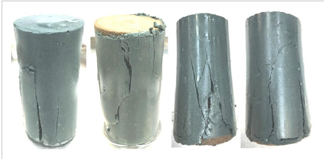
Figure 4.36: Failure modes at 60 days of curing in TXUU tests. Note that the colours were adjusted for better visibility.
