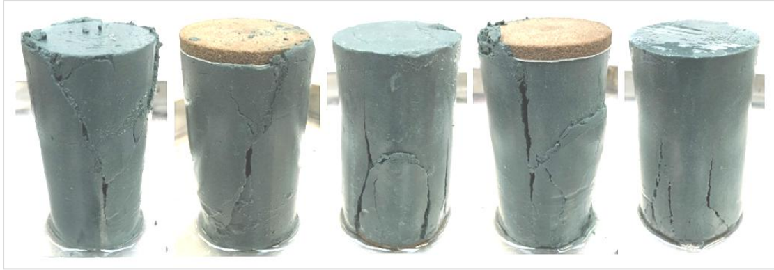
Figure 4.24: Failure modes at 30 days of curing in TXUU tests. Note that the colours were adjusted for better visibility.
