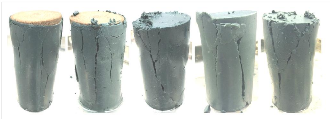
Figure 4.48: Failure modes at 90 days of curing in TXUU tests. Note that the colours were adjusted for better visibility.
