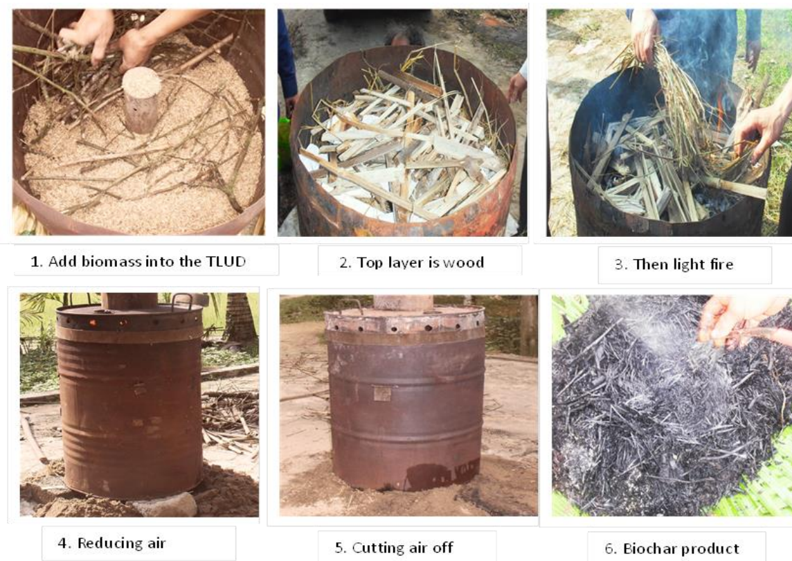
Figure 2.3. The pyrolysis process for biochar production using the TLUD equipment.
