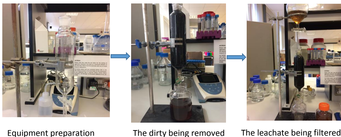
Figure 2.5. Conducting the biochar filter for the landfill leachate.
