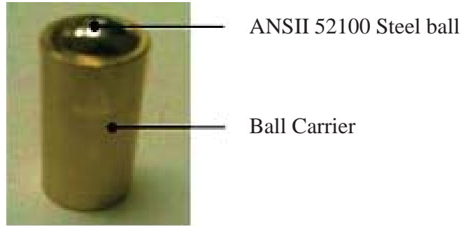
Figure 3-4: Ball carrier: 6mm ANSI Steel ball secured into ball carrier by means of an interference fit.
