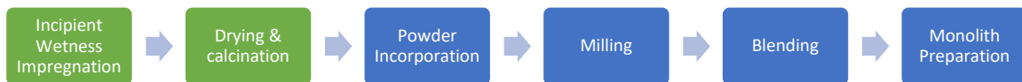
Figure 6-1: Process flow diagram for catalyst preparation with incipient wetness impregnation steps added (green)
