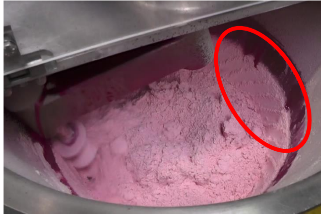
Figure 6-30: Nauta mixer after final addition of liquid with layer pressed between screw and wall highlighted
