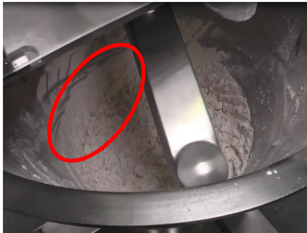
Figure 6-29: Nauta mixer before addition of liquid with layer pressed between screw and wall highlighted
