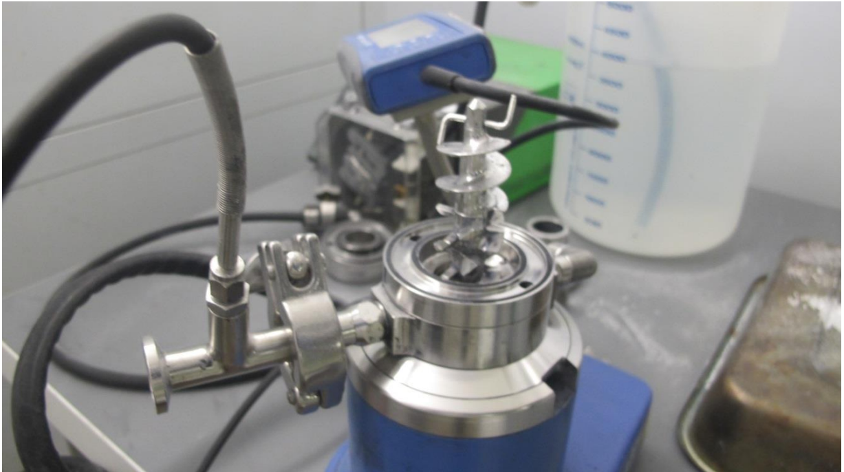
Figure 4-6: Photo of IKA MagicLAB MHD head moving parts
