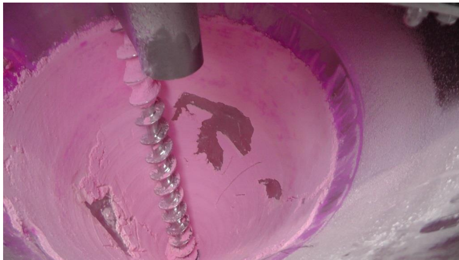
Figure 6-30: Nauta mixer after final addition of liquid with layer pressed between screw and wall highlighted
