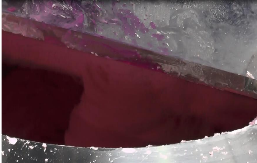
Figure 6-32: Powder stuck to CPM shaft
