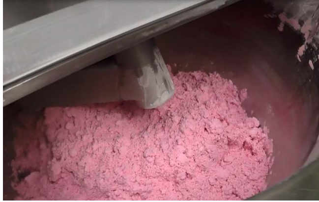
Figure 6-34: Nauta mixer after impregnation with wall > 60oC after stuck layer collapsed
