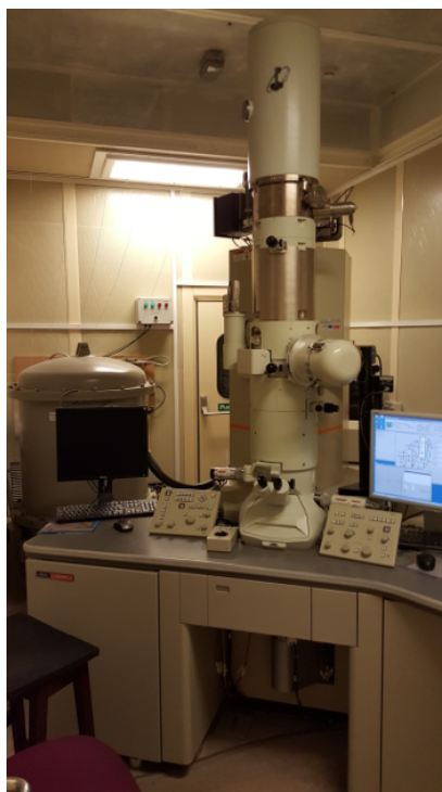
FIGURE 3.5: The C_s corrected JEOL 2100F STEM, capable of producing 200 keV electron beam.
