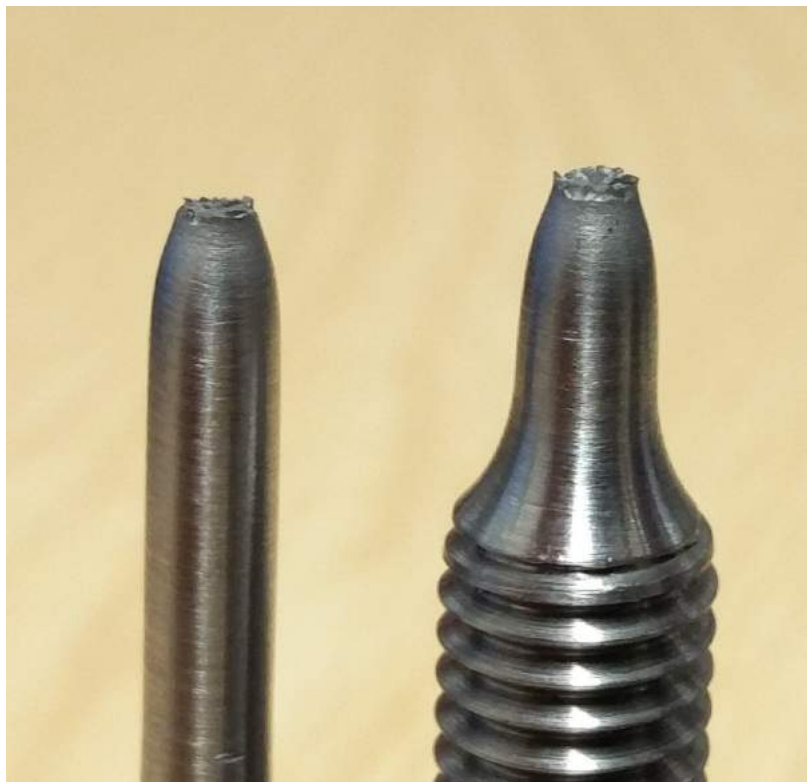
Figure 4.24: 24U3 sample showing ductile fracture (cup-cone).
