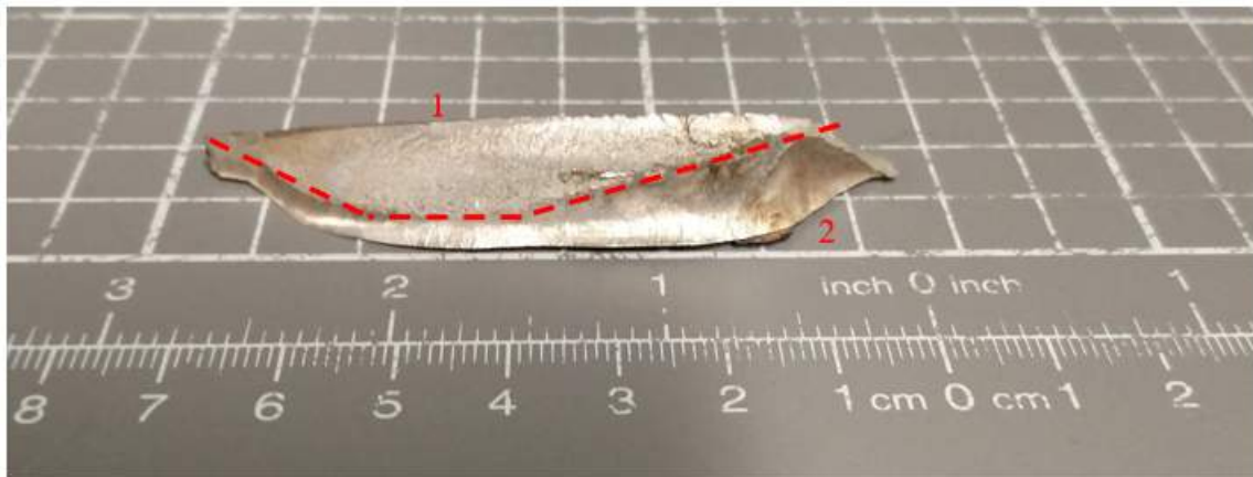
Figure 6.7: Bottom of broken tooth. Each square has a side of 1 cm.
