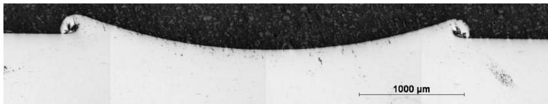
Figure 5.13: Optical micrograph showing cross-section of the wear track of the untreated fully lubricated sample.
