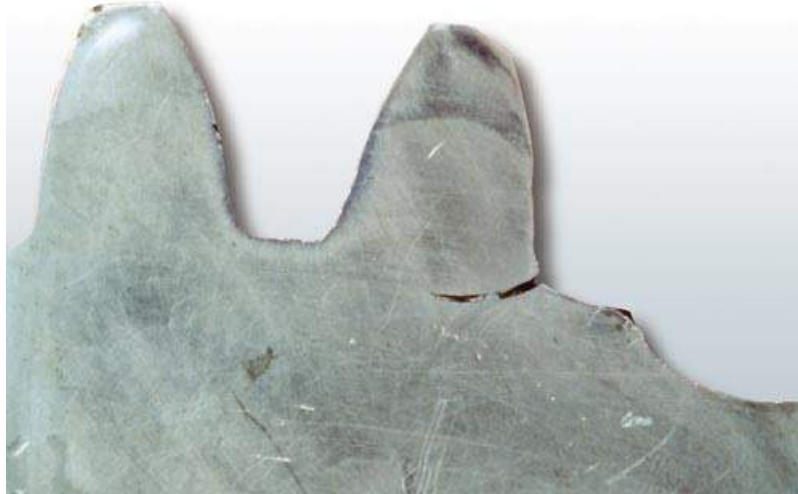
Figure 2.9: Tooth bending fatigue crack of a spur gear. Source: [54].
