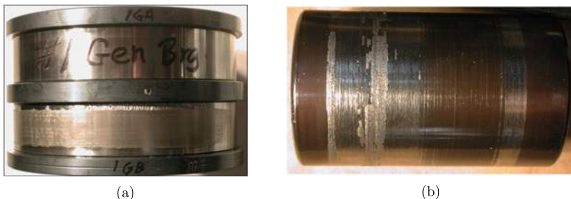
Figure 2.6: Micropitting in the inner race of a bearing (a). Scuffing in bearing roller (b). Source: [49].
