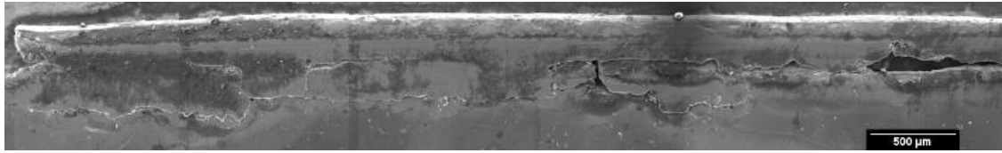
Figure 5.19: SEM micrograph of the wear track of the untreated dry-lubricated sample after 2 million cycles.
