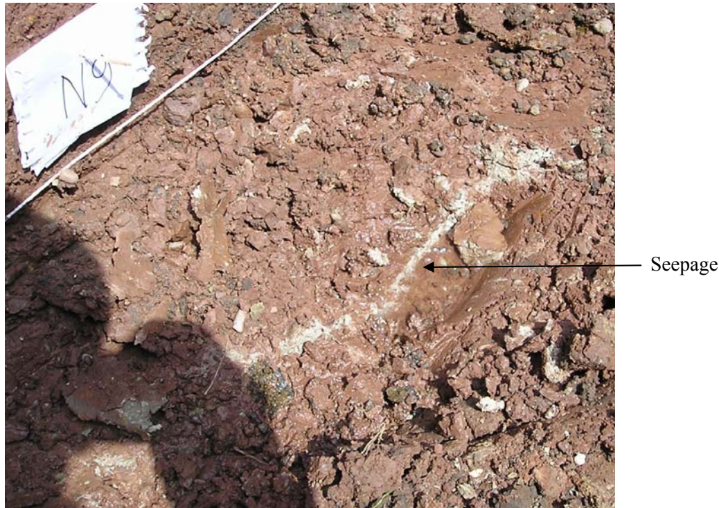
Figure 5.33 Photograph showing seepage from fracture in base of test pit
