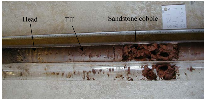
Figure 3.16 Core from borehole S1_1 showing head, lodgement till and a sandstone cobble
