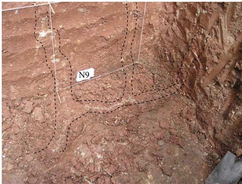
Figure 5.30 Photograph showing the connectivity of fractures in north face and base of test pit
