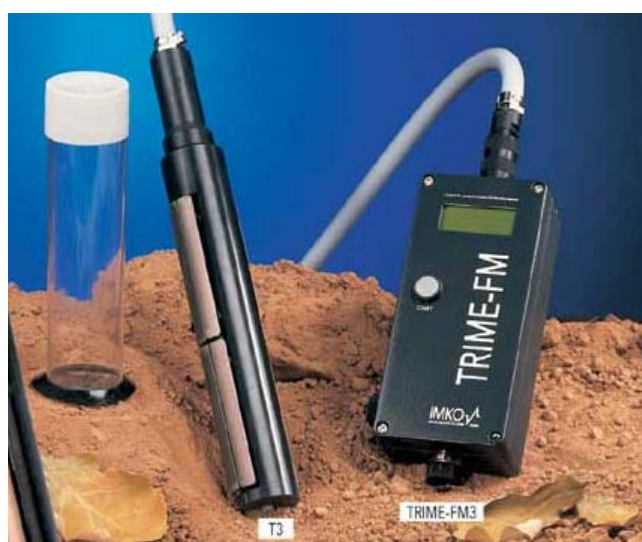
Figure 4.5 TRIME TDR T3 probe and access tube
