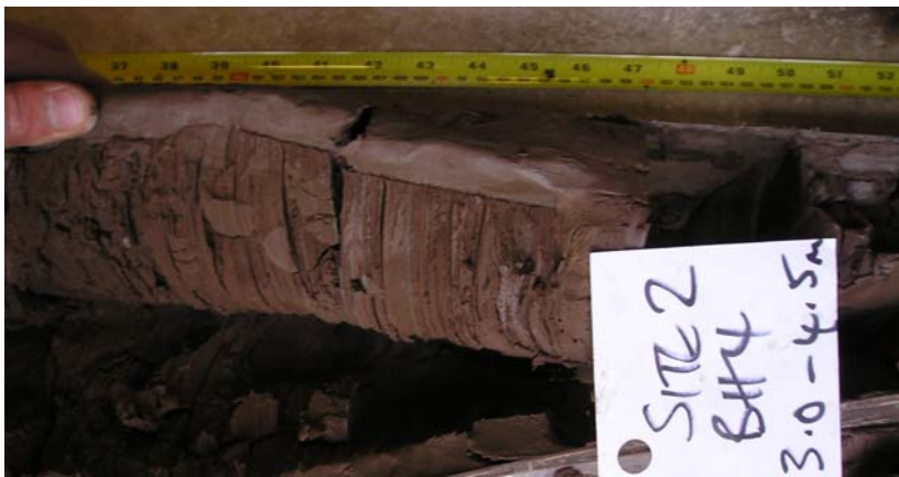
Figure 3.21 Laminations in glaciolacustrine clay within core from borehole S2_4
