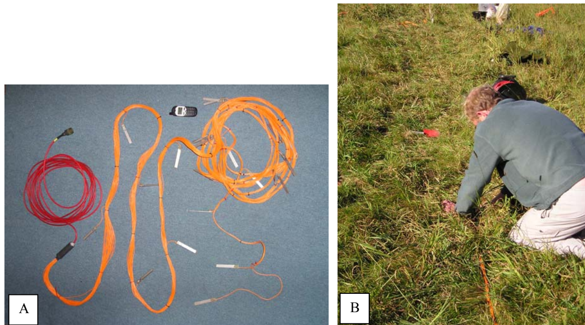
Figure 4.6 Permanent ERT array (A) being installed (B)
