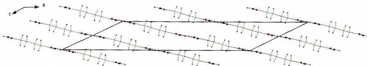
Figure 5.7.12: End-on view of adipamide (form I) structure 2 showing the adipamide sheets along the (101) plane within.
