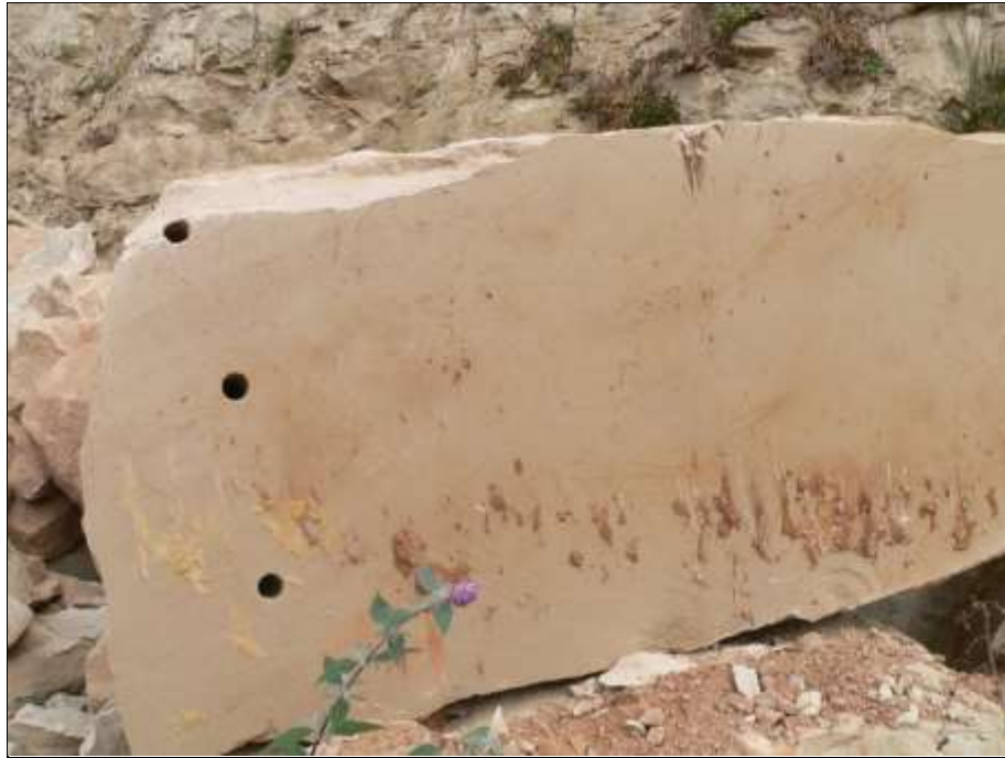
Figure 5: Block of stone extracted by use of Bristar Powder. Taken by author 10/08/2011.
