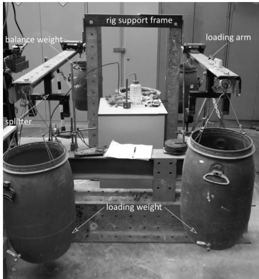
Figure 3.7. Initial loading arrangement for PS1, including lever arms for load transfer to a soil sample
