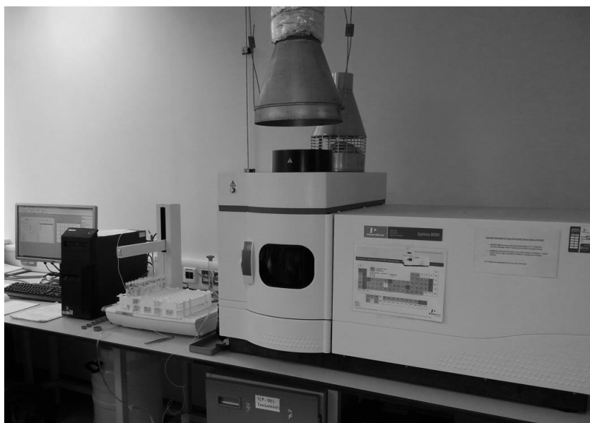
Figure 3.18. ICP-OES testing: (a) sample filtration; (b) storage of the samples; and (c) sample testing using the Perkin Elmer Optima 8000
