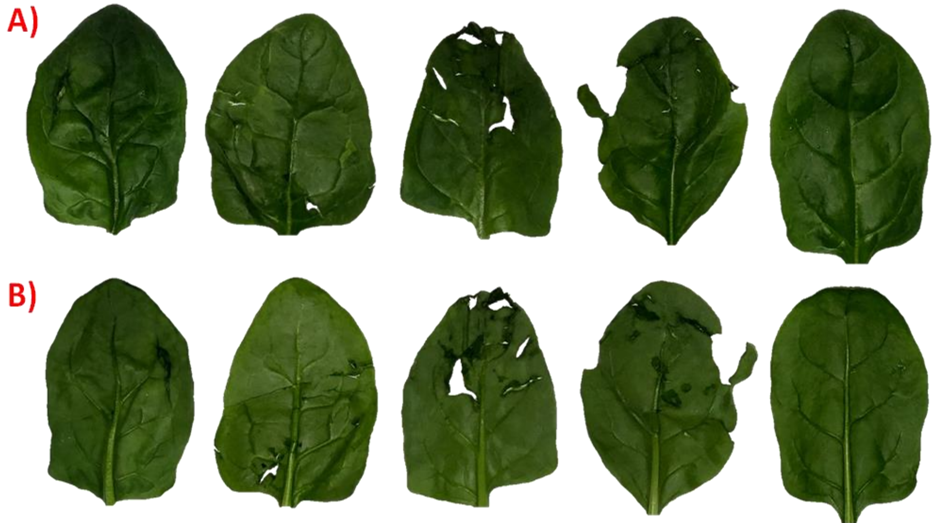
Figure 4.10: Digital images showed mechanical damage of Baby spinach leaves after 200N compression A) Front sides; B) Back sides.
