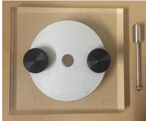
Figure 3.4: Penetration rig and probe.
