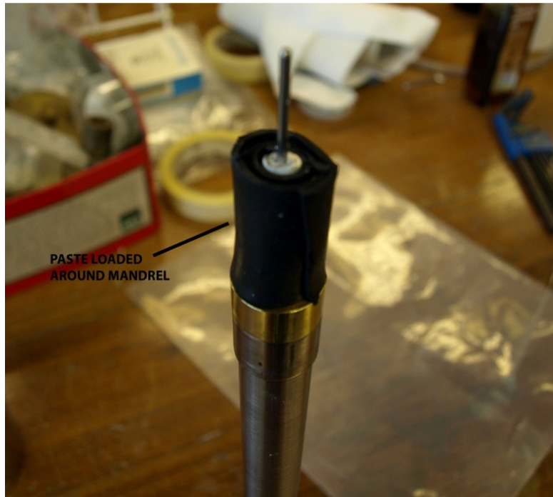
Fig.29. Pastes wrapped around mandrel of ram.
