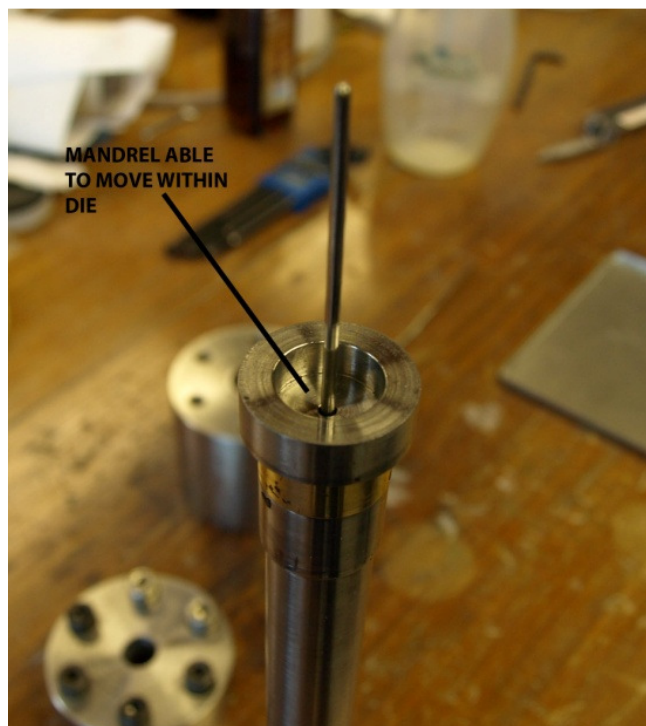
Fig.31. Mandrel through die without brass collar.
