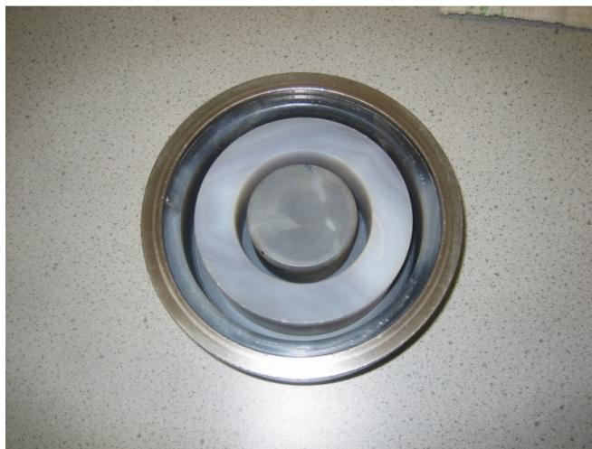
Fig.25. TEMA mill showing internal rings 39
