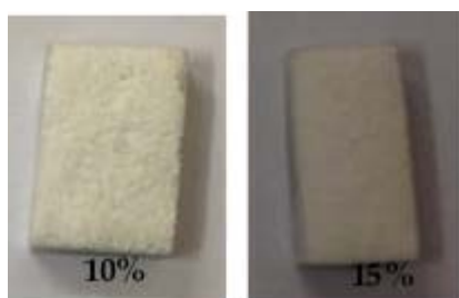
Fig. 5-64 Aluminium fumarate coated samples with 10wt% and 15wt% binder for microhardness test.
