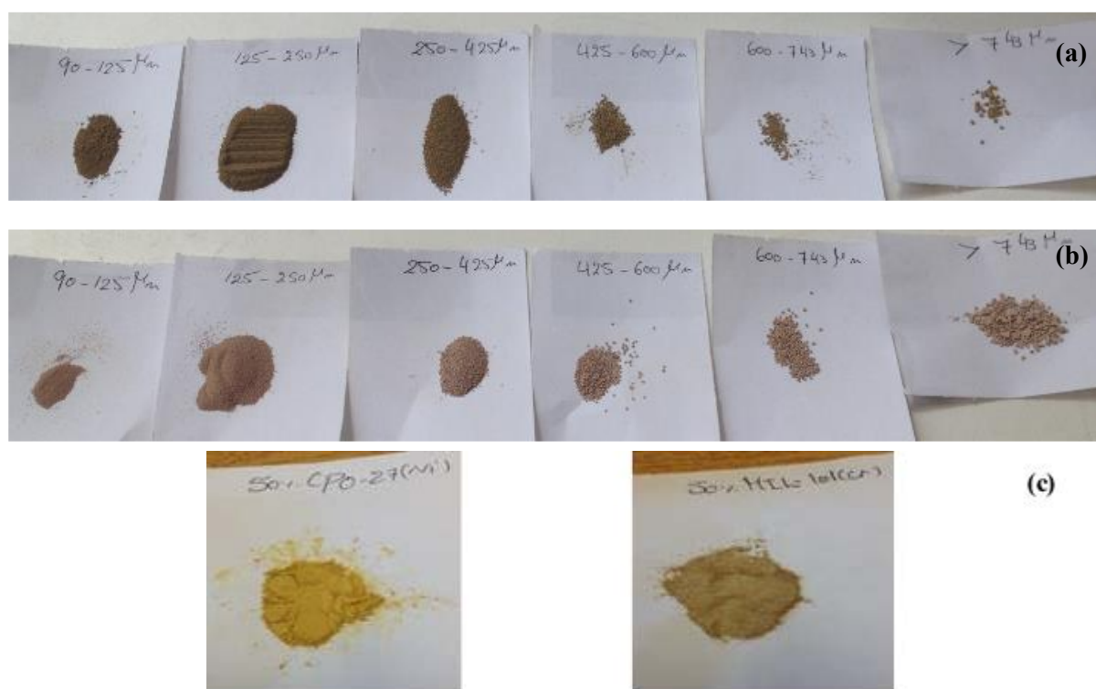
Fig. 5-75 MIL-100(Fe) composite: a. synthesized CPO-27(Ni)/MIL-100(Fe), b. synthesized MIL-101(Cr)/MIL-100(Fe) and c. physical mixture of CPO-27(Ni)/MIL-100(Fe) and MIL-101(Cr)/MIL-100(Fe).
