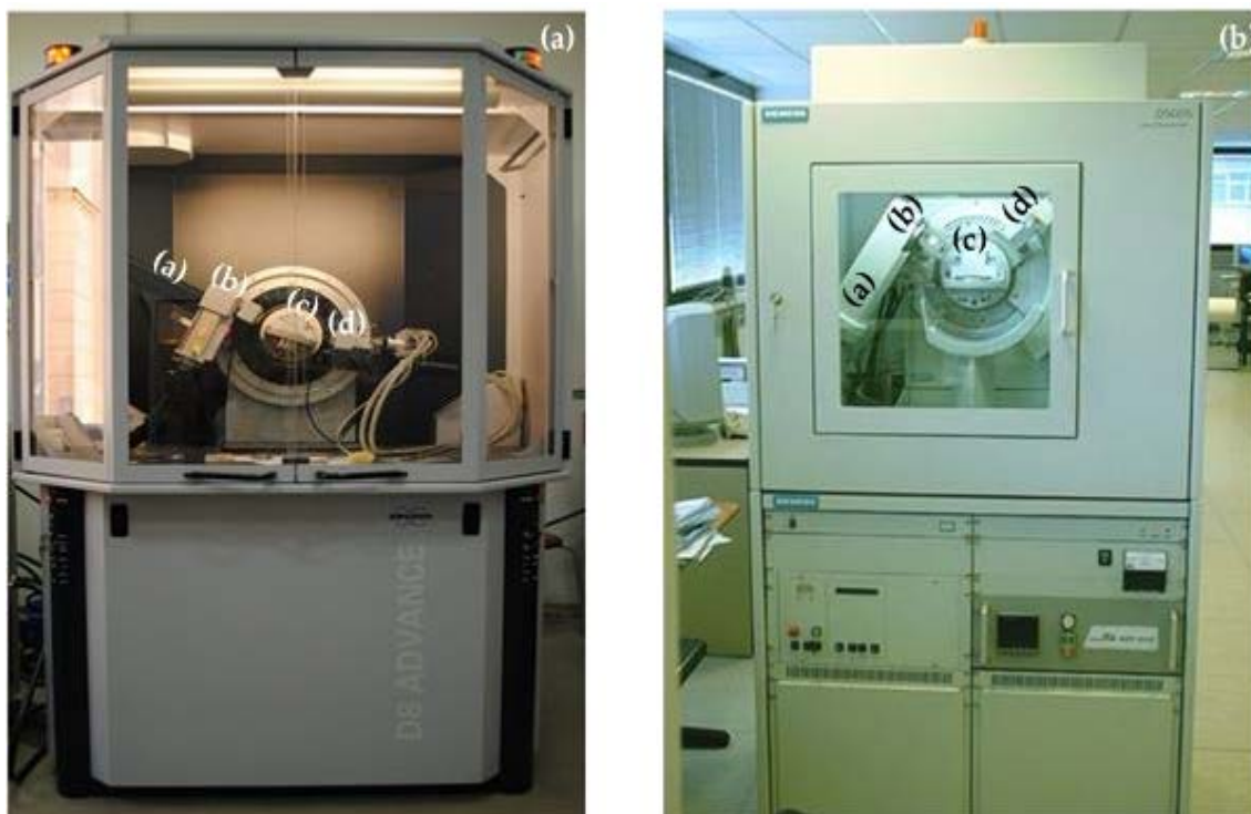
Fig. 3-3 a. D8 Advance-Bruker and b. Siemens D5005. ((a) X-ray source, (b) monochromator, (c) sample holder and (d) detector).
