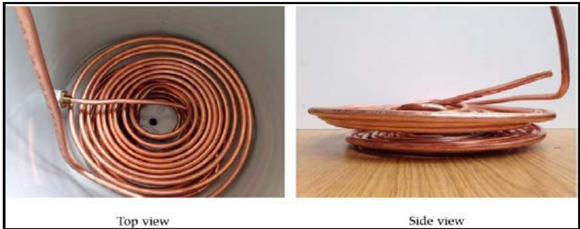
Fig. 7-3 Top and side views of the copper coil in evaporator.
