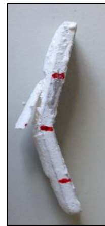
Fig. 5-73 Images of substrate, 10wt% binder sample before and after three points bending test.
