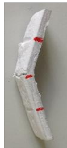
Fig. 5-73 Images of substrate, 10wt% binder sample before and after three points bending test.
