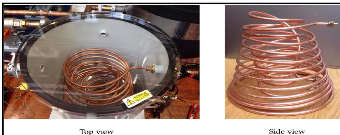
Fig. 7-5 Top and side views of the copper coil in condenser.
