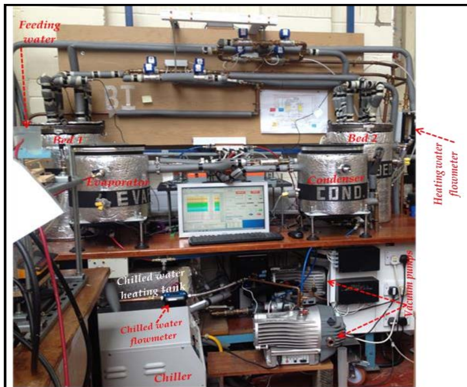
Fig. 7-1 Schematic diagram and pictorial presentation of the 2-bed system test facility.
