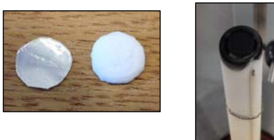
Fig. 5-61 Substrate, aluminium fumarate coated sample and graphite plated sample in furnace for thermal conductivity measurement.
