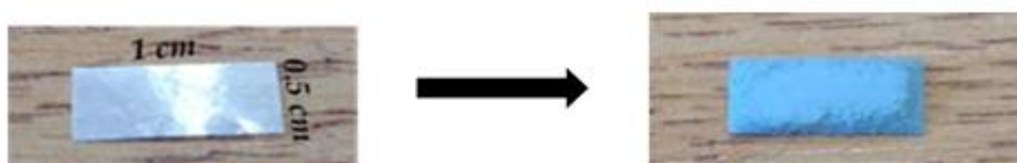
Fig. 5-52 Metal substrate before and after coating with MIL-101(Cr).
