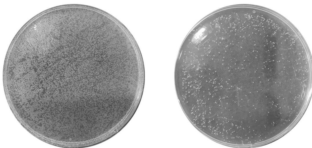
Figure 4. 57 P. gingivalis colonies on the soya agar plates after 5 h contact with (a) glass and (b) Ag impregnated composite coating
