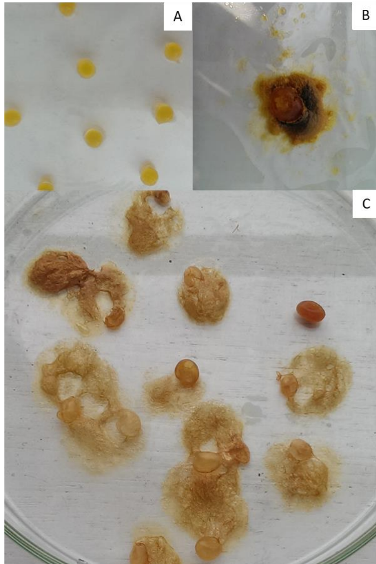
Figure 5.5 “nanopopcorn” beads containing \text{Fe}(\text{NO}_3)_3 and starch A - pre microwave, B - 30 second in 700W microwave, C - 1 min in 700W microwave.
