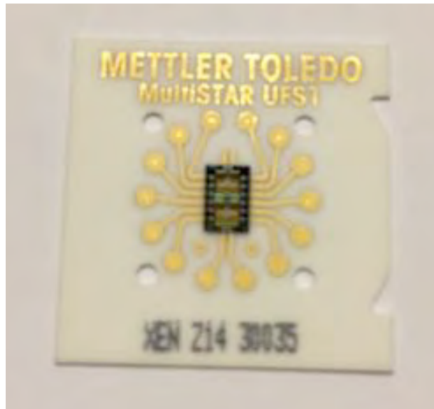
Figure 2-11: MultiSTAR chip sensor from Flash DSC1.
