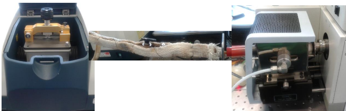
Figure 97: FTIR connected with the Exstar 6000 TGA with heated transfer line.
