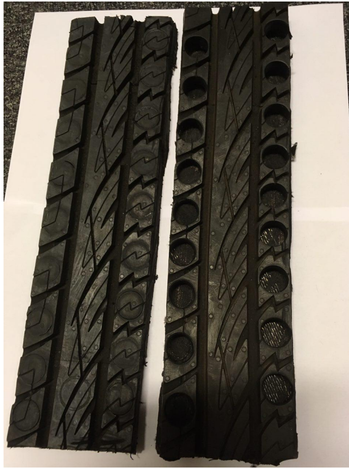
Figure 4-1 Sample preparation progress-a) tread was separated from the tyre sidewalls with grinders-b) a pin sized samples were drilled/punched into the tread c) tread was separated from the reinforcement by hack-saw, so the pin could be extracted
