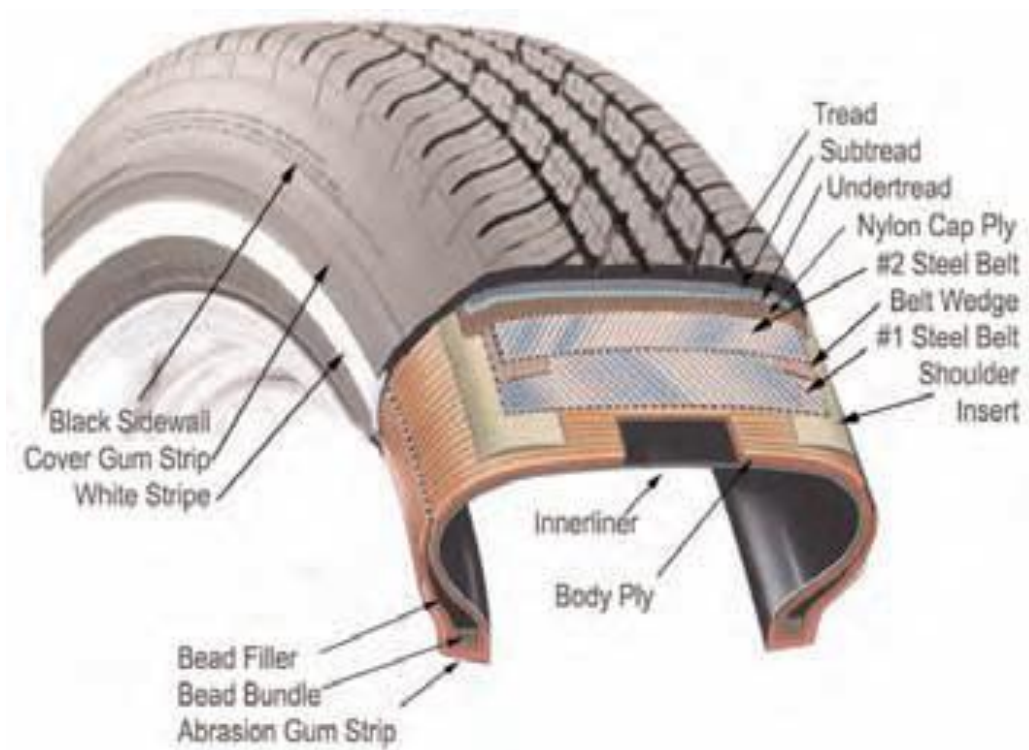
Figure 2-23 Tyre cross section [60]
