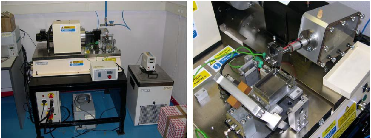
Figure 2-20 Flat on flat and flat on cylinder contacts in TE77 tribometer [59]
