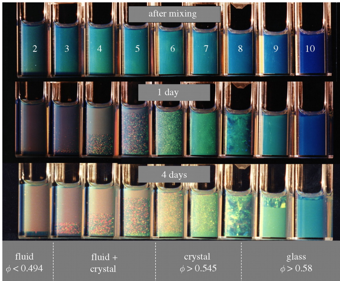
Figure 1.5: The phase behaviour of hard-sphere colloids. 77 Adapted with permission from the Royal Society.
