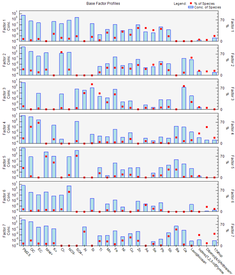
Figure 4-5 Factor profiles when seven factors was set before the model run
