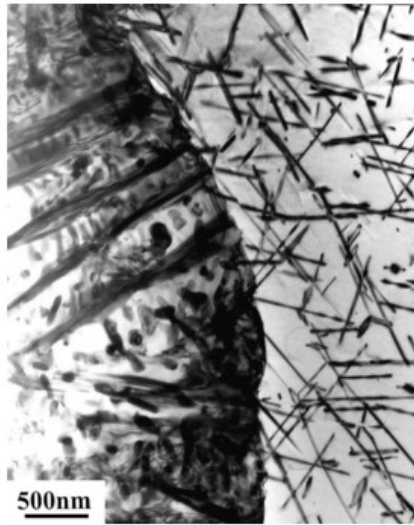
Fig. 2.4 Morphology of Mg_{17}Al_{12} discontinuous precipitate[66]
