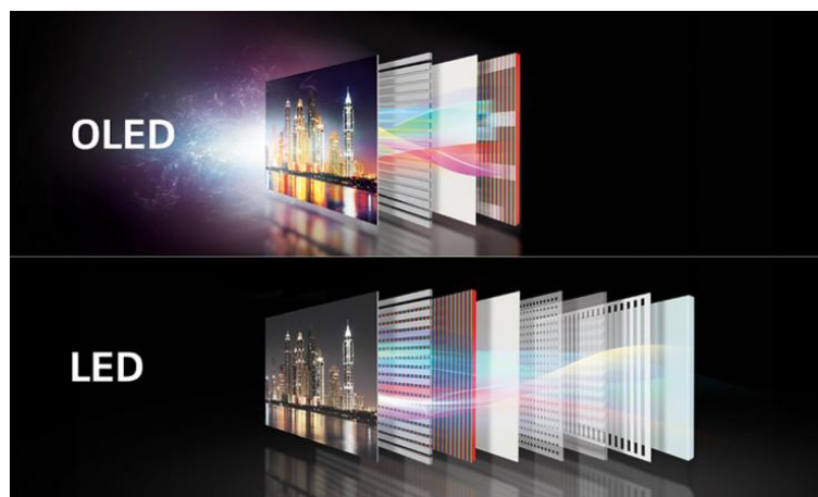
Figure 1.1: Figure to show the comparison between OLED and LED television. 8
