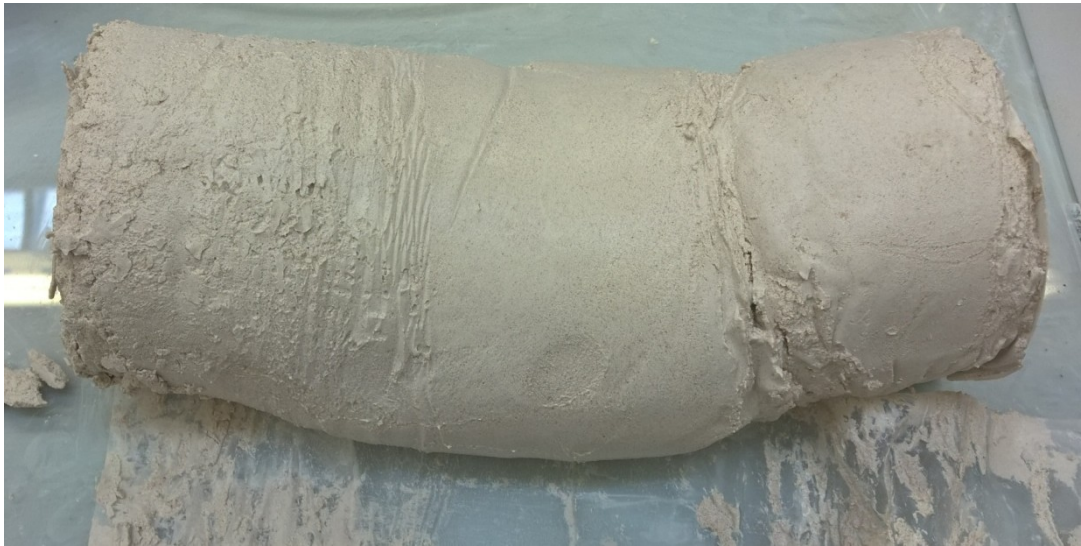
Figure 4.10: Central wet zone in a consolidated sample (a sleeve is used but does not extend to include the top cap). Localised lower strength is apparent from the central bulging.
