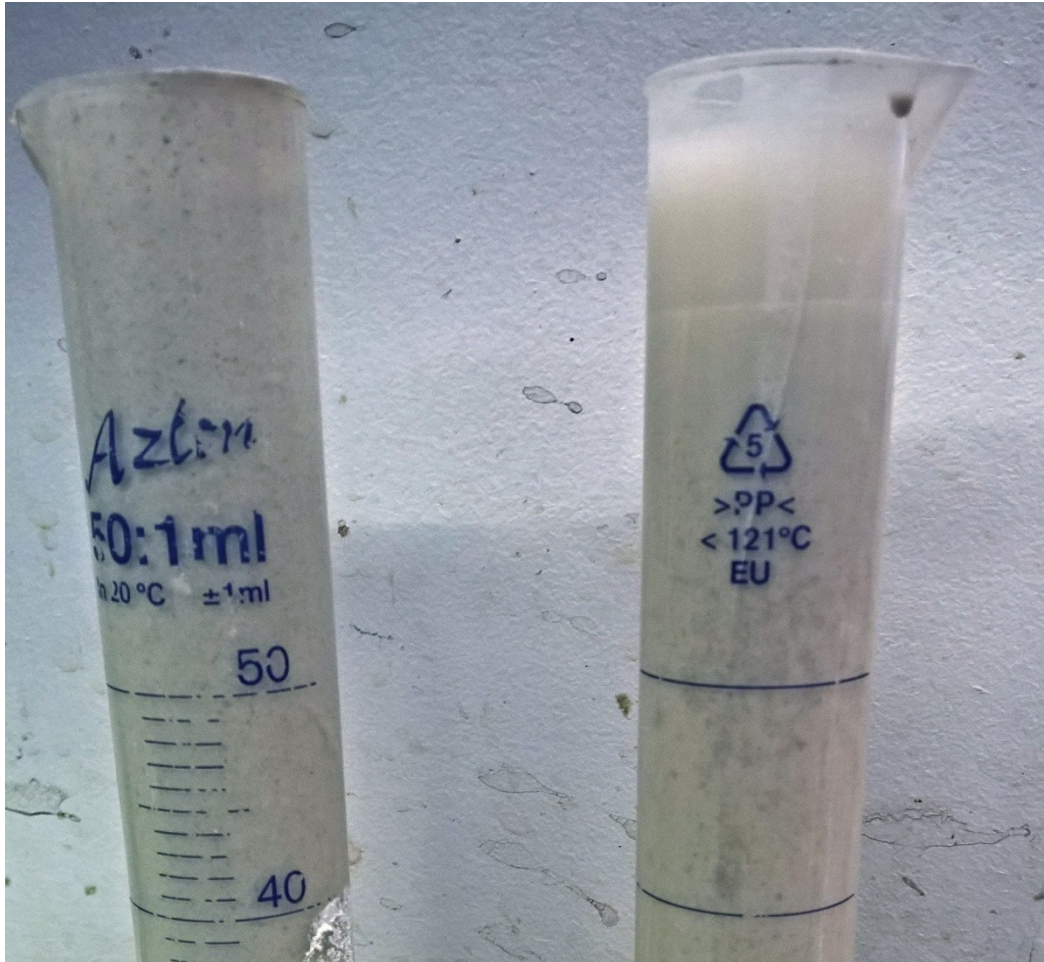
Figure 4.8: Silt mix slurry mixed and left to stand for 1 hour. Left – slurry mixed at 1.5 LL, relatively uniform. Right – slurry mixed at 2 LL, varying from thin suspension near the top to predominantly fine soil beneath, becoming coarser at depth.
