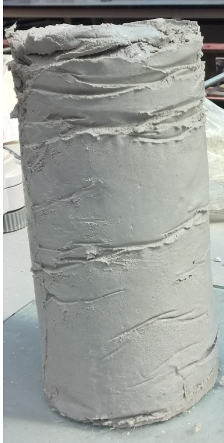
Figure 4.12: Creases in a soil sample consolidated using a polythene sheet as a compressible sleeve
