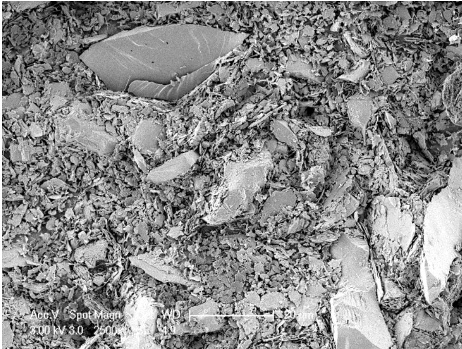
Figure 4.19: Micrograph on horizontal cut plane of under-compacted Silt Mix soil illustrating random alignment similar to Figure 4.18.
