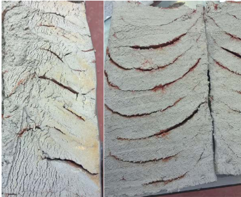
Figure 4.6: inclined compaction surfaces highlighted by adding red ink between layers. The sample is constructed from bottom to top. Left – heavy compaction, convex surfaces. Right – light compaction, concave surfaces.
