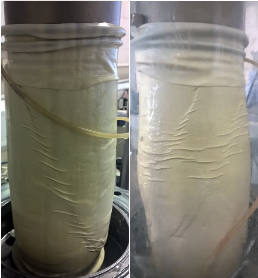
Figure 4.45: Differences in triaxial sample failure mode as a result of top lubrication: left - standard ends and single slip, right - lubricated top and multiple slip planes.
