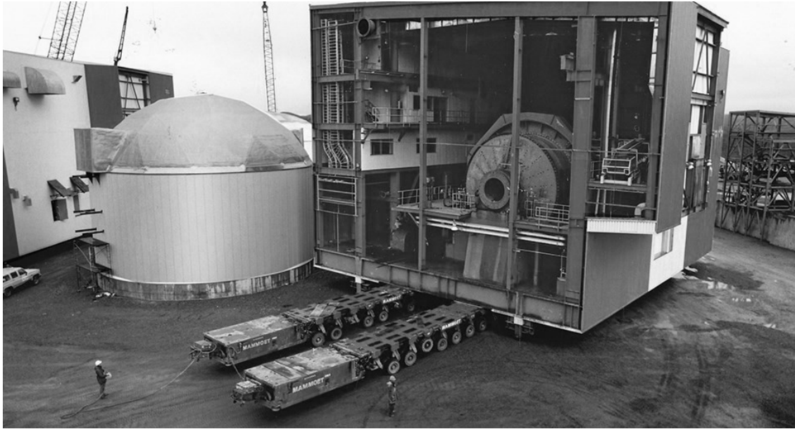
Figure 1.1: Heavy equipment being transported on a platform composed of Self-Propelled Modular Transporters (SPMTs), Courtesy of and ® of Mammoet BV.
