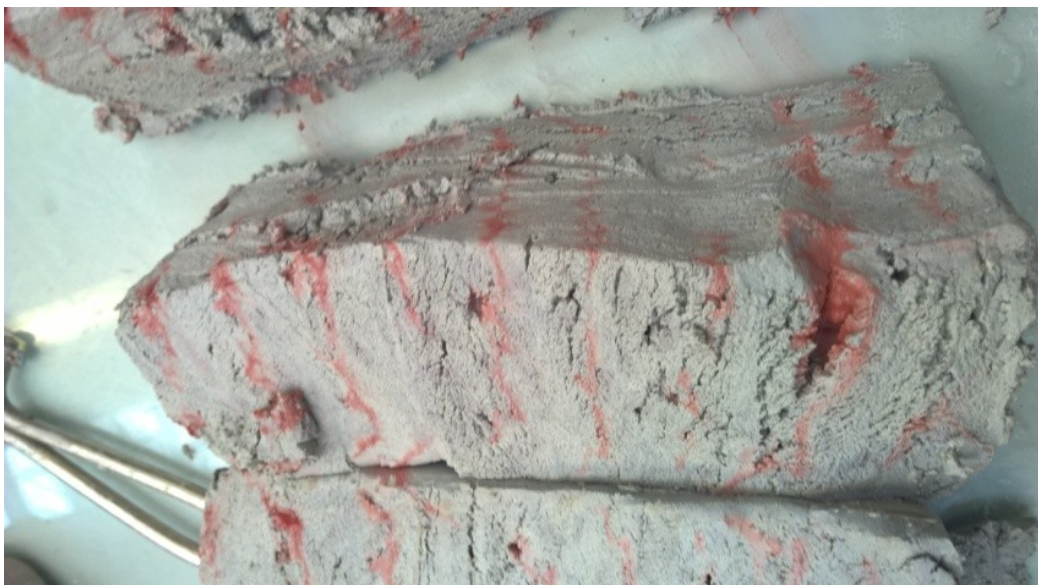
Figure 4.7: A sample following 'mixed' compaction: layers are approximately horizontal and evenly spaced.
