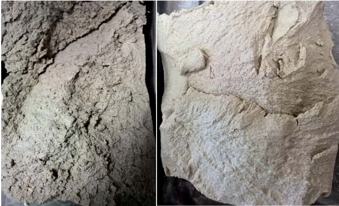
Figure 4.15: Internal fabric of 100mm diameter triaxial samples split in half vertically. Left - prepared using the under-compaction method. Right - prepared by slurry consolidation.
