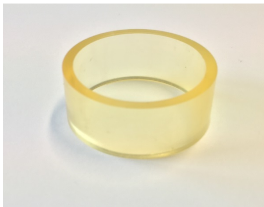
Figure 6.3: Polyurethane ether sheath used in the first assembly.
