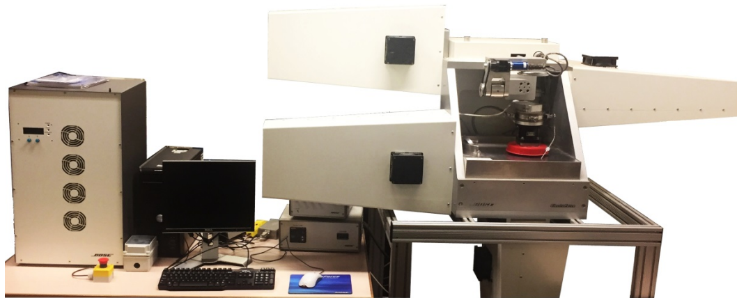
Figure 6.9: Bosc spine simulator SDWS-1 Simulator, with multi-axial AMTI MC3-6-1000 load.
