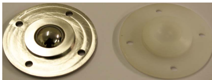
Figure 6.1: CoCr ball and UHMWPE socket.
