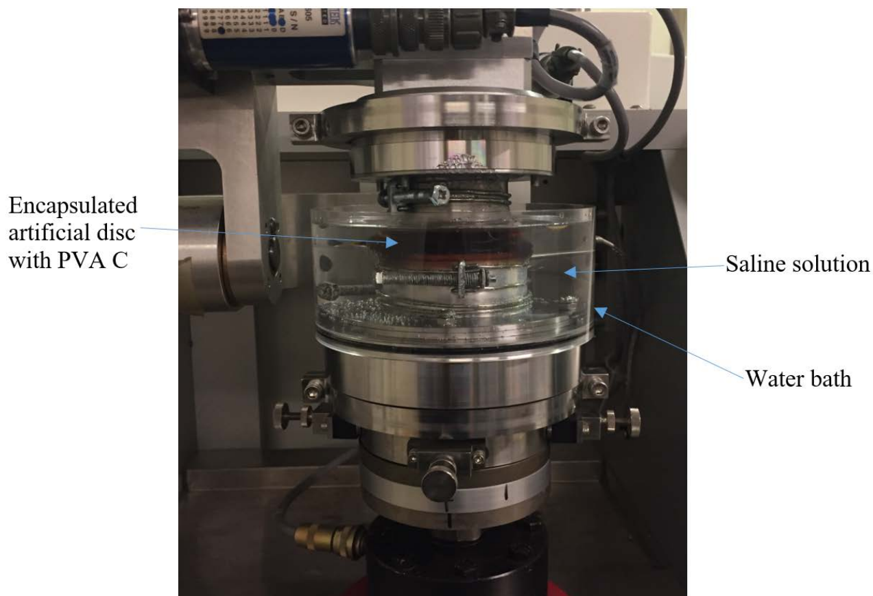
Figure 7.3: The assembly configuration 5, mounted on the Bose spinal simulator. The sheath is fixed using a double wire hose clamp, the PVA C lubricant contains a red dye and the whole device is surrounded by saline solution (9.5 g/L of sodium chloride in deionized water).
