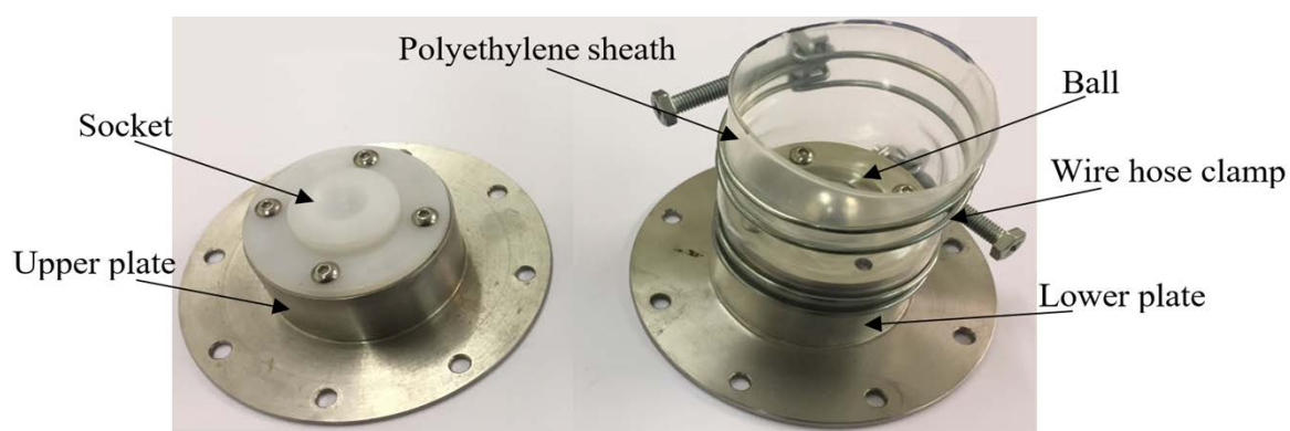
Figure 7.2: The ball attached to the polyethylene heat shrink sheath and the lower plate using a double wire hose clamp before inserting the lubricant.
