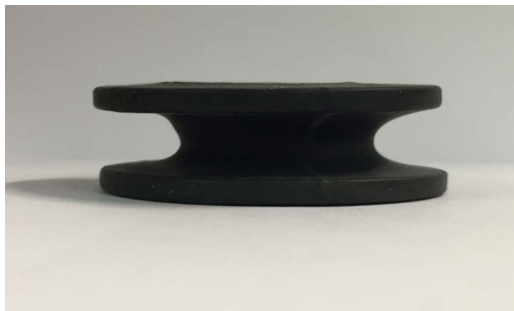
Figure 6.7: Butyl rubber attached to the ball and socket artificial disc using Super glue all plastics.
