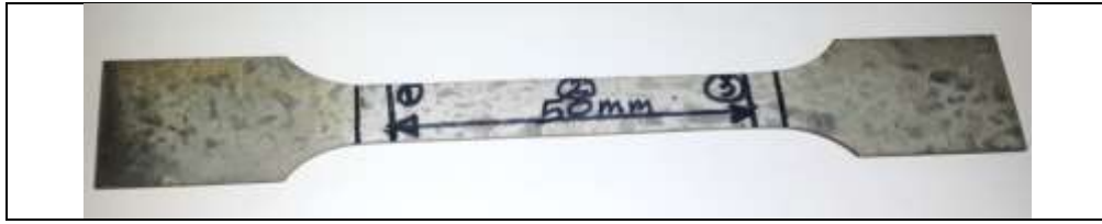
Figure B.3 Specimen geometry- all dimensions in mm
