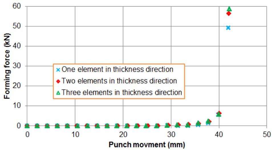
Figure 4.8 Punch force distribution in Y-direction with different numbers of mesh elements in the thickness direction of sheet
