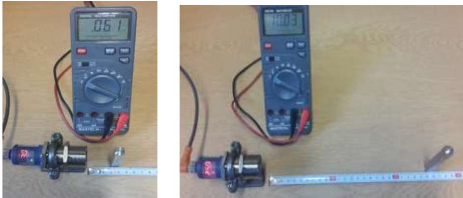
Figure 6.21 Distance transducer calibration using voltmeter
