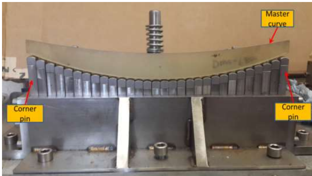
Figure 6.20 Pin adjustment using master curve
