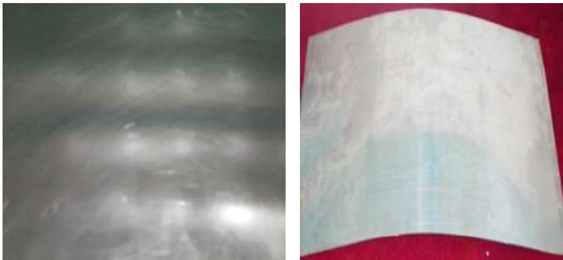
Figure 2.22 Dimpling (a) clear dimpling, and (b) no dimpling using 10 mm pin size [20]
