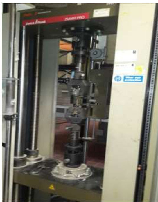
Figure B.1 Tensile test machine in Metallurgy and Materials Department at the University of Birmingham
